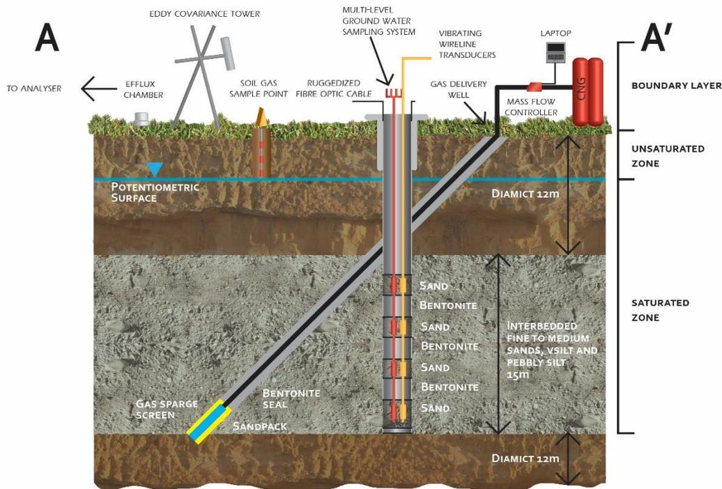
Figure 2. Cross-section A-A' (see Figure 1), showing the natural gas release system and the monitoring infrastructure in the saturated, unsaturated, and atmospheric layers (Cahill et al., 2019).
