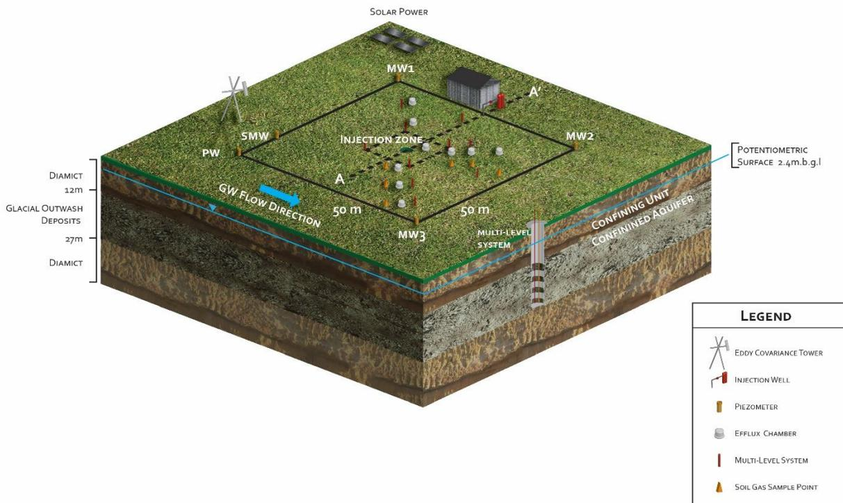
Figure 1. Conceptual model of HHFRS and the controlled natural gas release experiment infrastructure, as well as the subsurface geology of the site (Cahill et al., 2019).
