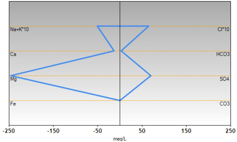
Figure 1. Stiff diagram for one the water samples.
