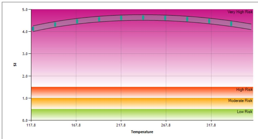
Figure 2. Saturation index versus temperature for dolomite scaling demonstrating the potential risk of scaling
