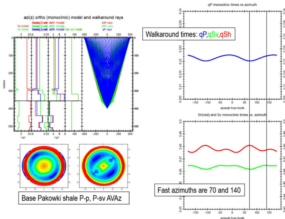
Figure 2. Upscaled monoclinic model with depth-dependent fast azimuth (upper left) and qP, qSv qSh rays from surface to a receiver at depth  $z=400\text{m}$  below the orthorhombic Lea Park formation. Lower left: Right: walkaround qP, qSh and qSv times for a circle at radius  $r=500\text{m}$ .
