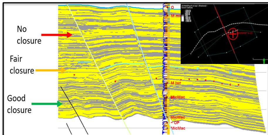
**Figure 5. A modelled cross section of the migrant structure populated with sand and shale properties from shale volume calculation. The figure shows the magnitude of crestal faulting through the offset of sand-shales.**
