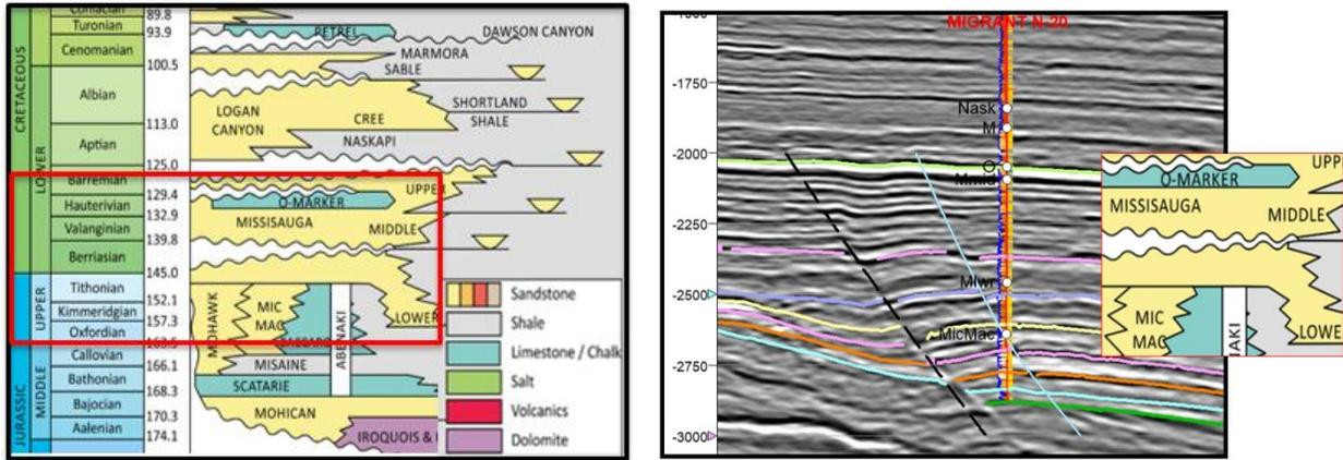
Figure 2. (Left) Lithostratigraphic chart of the Scotian Basin showing the interval of interest outlined in red (Weston et al. 2012). (Right) A seismic profile showing the Migrant rollover with the N-20 well penetrating the structure with interpreted horizons.
