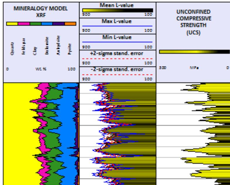
Figure 2. High UCS observed in zones of increased dolomite content and lower UCS in clay-rich zones.
