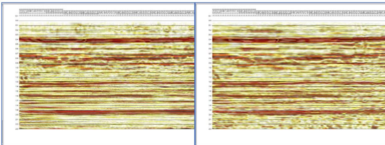
**Figure 2:** Final migrated stacks for dynamite (left) and Vibroseis (right) tests.
