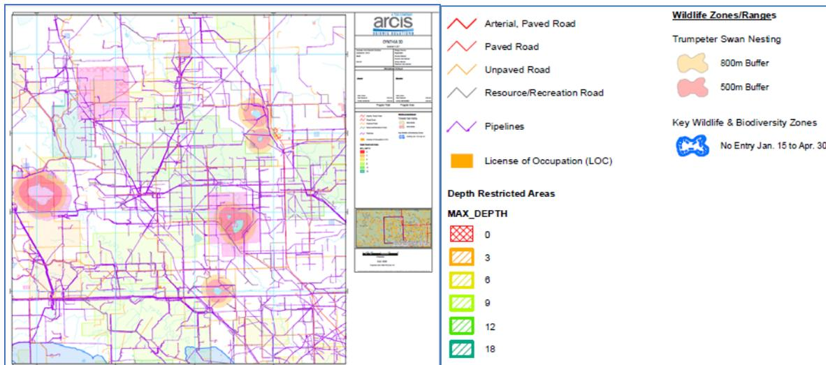
**Figure 1:** Map showing drilling-restricted areas (colored polygons) and setback-inducing infrastructure (colored polylines). 2D test line runs north-south in the middle of the map. Detailed legend provided at right.
