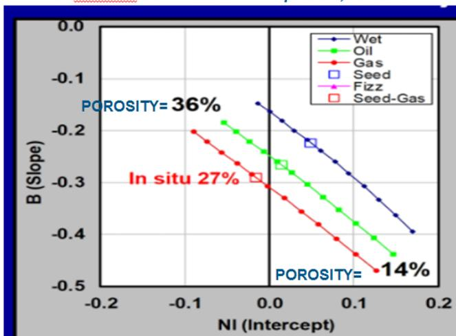
Figure 1. When lithology contrast (here, low impedance shale over high impedance sandstone) and pore fluid are held constant, the effect of increasing porosity is to decrease the Normal Incidence (Intercept) amplitude and cause the AVO gradient (slope) to become less negative (that is, to become more positive).
