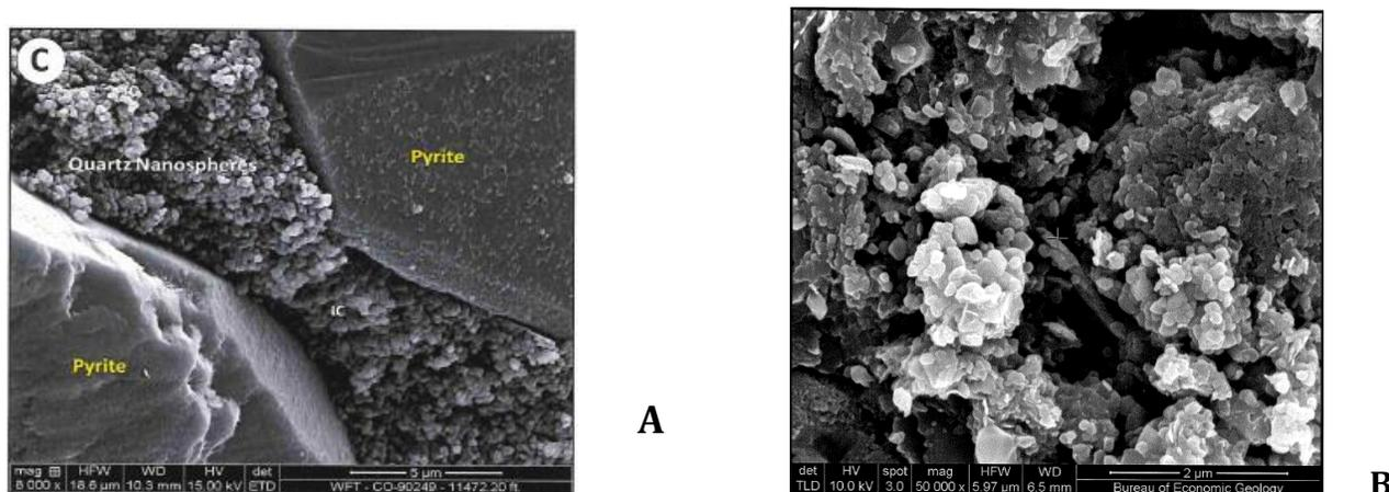
Fig. 1. SEM images of broken surfaces from Woodford (A) and Mowry (B) showing silica nanospheres of less than 0.5 micron diameter. From Longman et al., in press.
