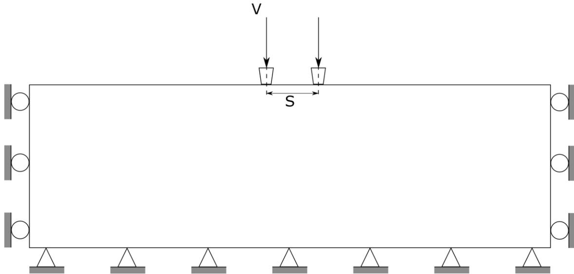
**Figure 1.** Geometry and constraints of the TBM disc cutters and rock sample. Rigid disc cutters are spaced by  $S$  using an  $s/p$  ratio and an enforced penetration rate,  $p$ . The velocity,  $V$ , is set to reproduce the vertical displacement of the cutter with a set penetration and cutter radius.
