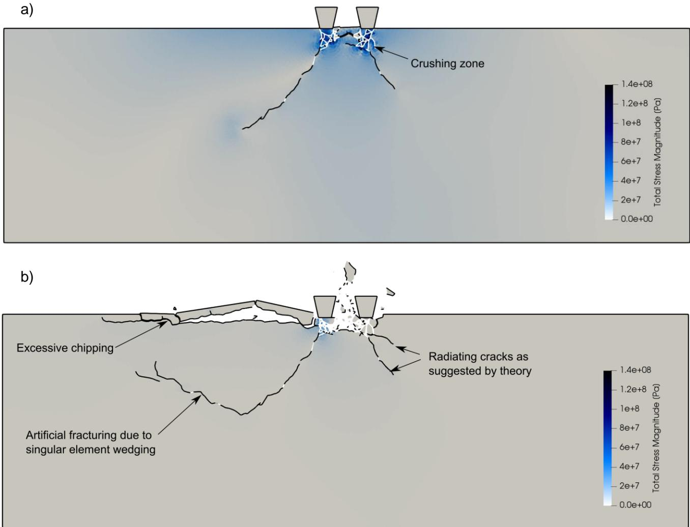
**Figure 2.** (a) Fractured model with  $s/p = 12$  and 4 mm penetration before crushing zone is expelled. The model extents and Mode I fracturing is shown in black. Mode II fracturing and Mixed Mode I-II is shown in white. The total stress magnitude is shown in blue. (b) Fractured model after the crushing zone is expelled.
