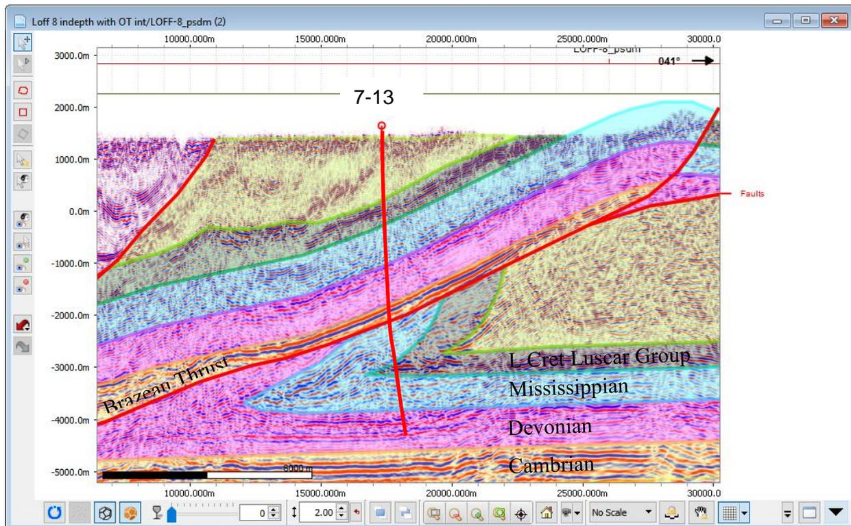
Fig. 2. Final PSDM depth section with 7-13 projected down plunge on to the plane of section.
