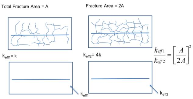
Figure 2. Simple model relating fracture area to effective permeability. As shown, doubling the total fracture area is equivalent to a 4x increase in effective permeability. However, the doubling of the effective permeability is equivalent to a 1.4x increase in total fracture area.
