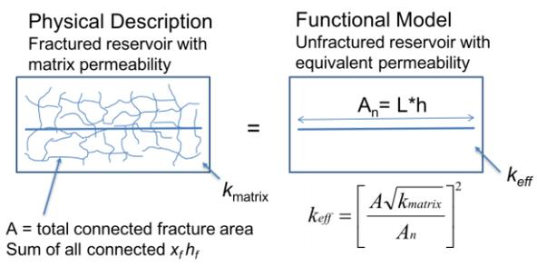
Figure 1. Schematic of fractured reservoir, where total area (A) is defined by the total connected fractures within the frac half length and width. And can be represented by a simple unfractured reservoir model with equivalent permeability to observed in the fractured reservoir. For unconventional shale play, the matrix permeability is negligible.
