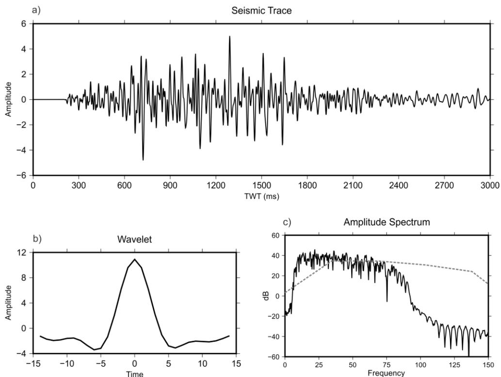
**Figure 1:** An example of wavelet estimation from stacked seismic data: a) seismic trace, b) estimated wavelet, and c) amplitude spectrum of the seismic trace (black curve) and of the estimated wavelet (grey dashed line).
