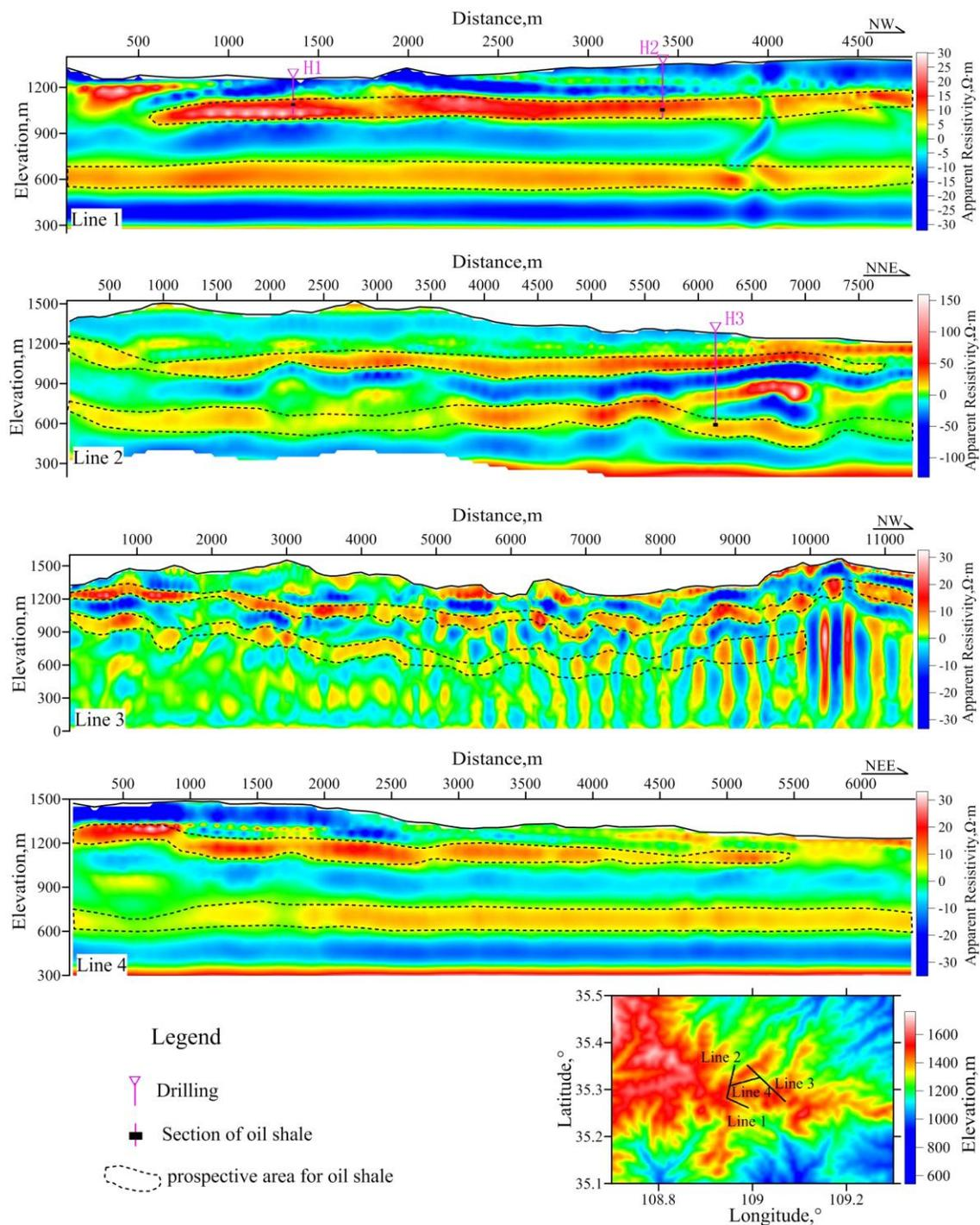
Fig. 2 High-pass filtered anomalies within the four apparent resistivity profiles of CSAMT for 2-D inversion. A filter with 400-meter geometric scale was selected.
