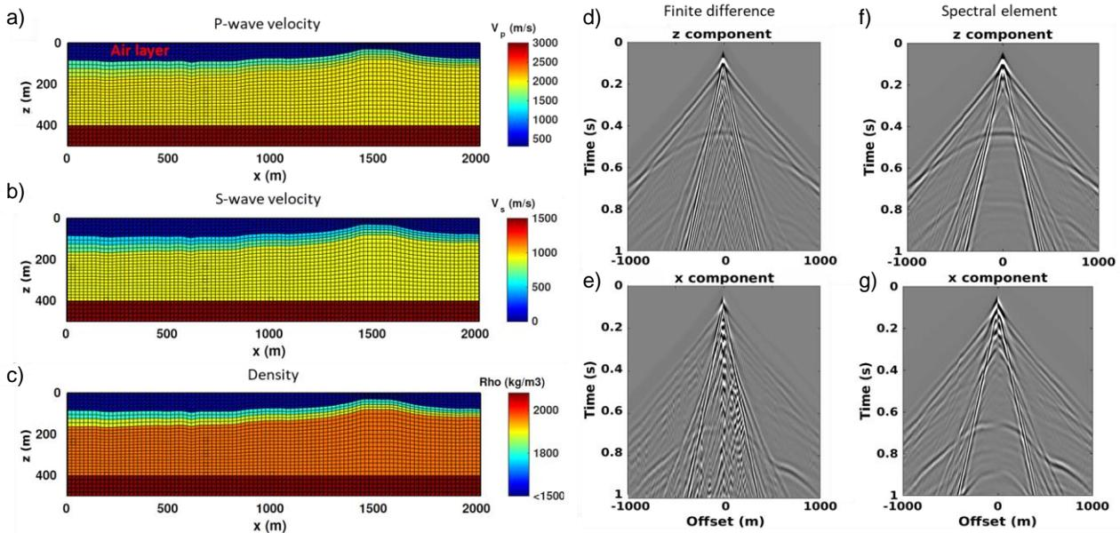
Figure 1. a) P-wave velocity, b) S-wave velocity and c) density models used to compute synthetic data. d) Vertical and e) horizontal component data computed using a finite difference algorithm. f) Vertical and g) horizontal component data computed using a spectral element algorithm.
