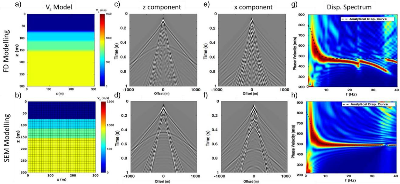
Figure 2. From left to right, near-surface velocity model used to compute synthetic data, vertical and horizontal component data obtained and the dispersion spectrum computed from the vertical component data. The top row are the results after using a FD algorithm and the bottom row shows the results with a SEM algorithm.
