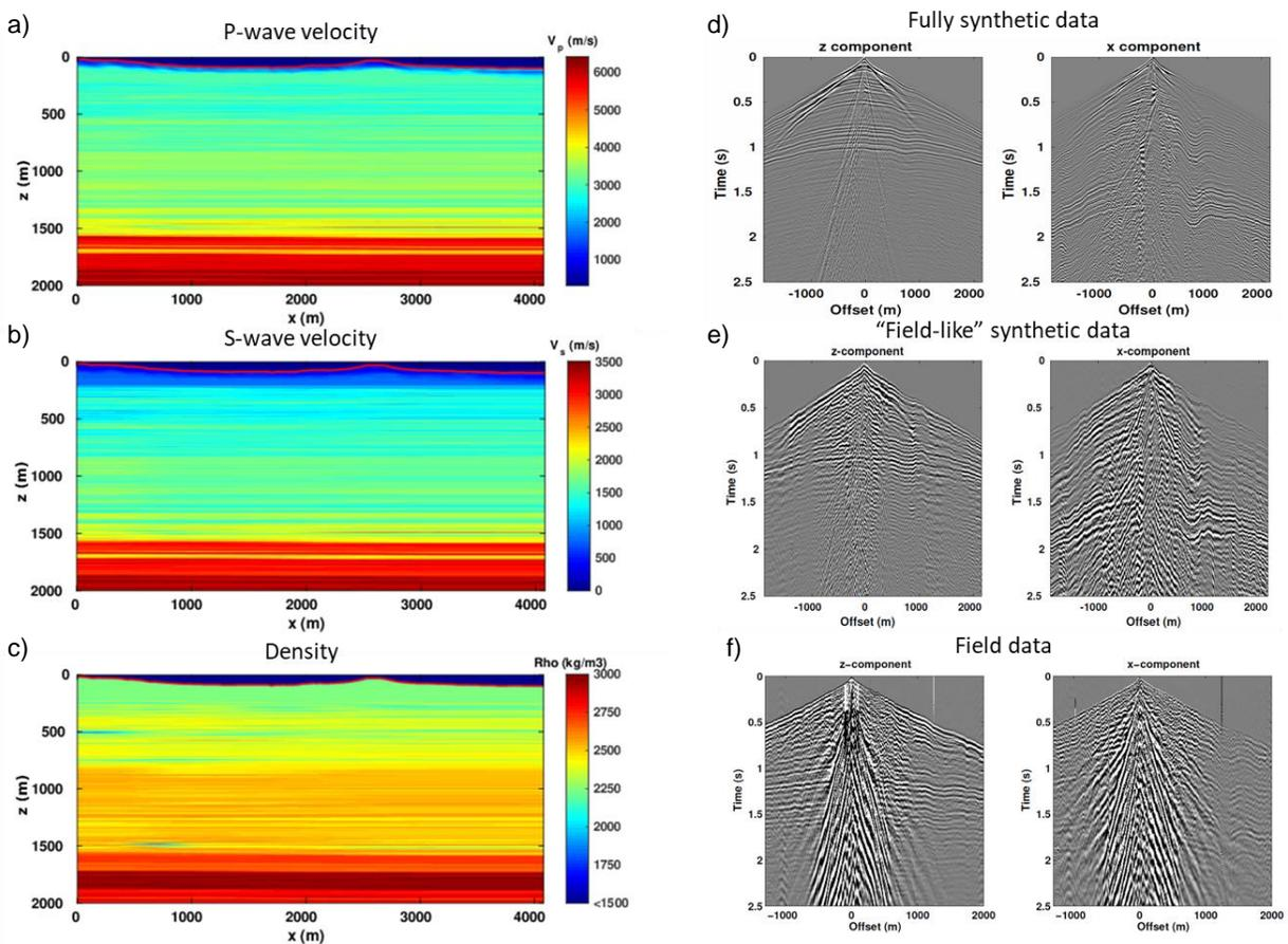
Figure 3. (a) P-wave velocity, (b) S-wave velocity and (c) density models generated with the well log data available along the Hussar 2D-3C seismic line and a tomographic near-surface velocity model. d) Fully synthetic source gathers and (e) “field-like” synthetic gathers obtained after imposing the surface-consistent effects observed in the real data. (f) Horizontal and vertical component data recorded on the field.
