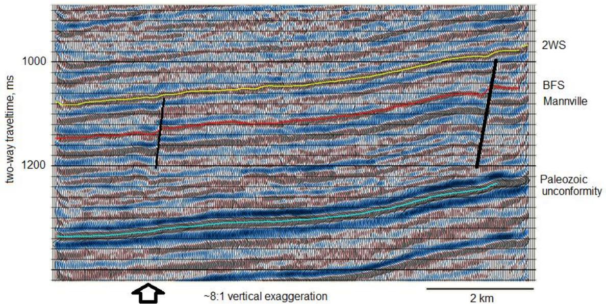
Figure 2. Image from a 3-D seismic dataset recorded in southern Alberta. Two normal faults are interpreted. The BFS marker is faulted down ~5 m across a ~300-400 m distance left of both fault traces. The Barons Sandstone reservoir is created and preserved in some of these faults.
