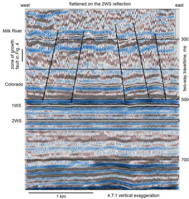
Figure 3. Image from a 3-D dataset near the Manitoba Saskatchewan border. The strata above the 2WS reflection are heavily faulted with growth faults.
