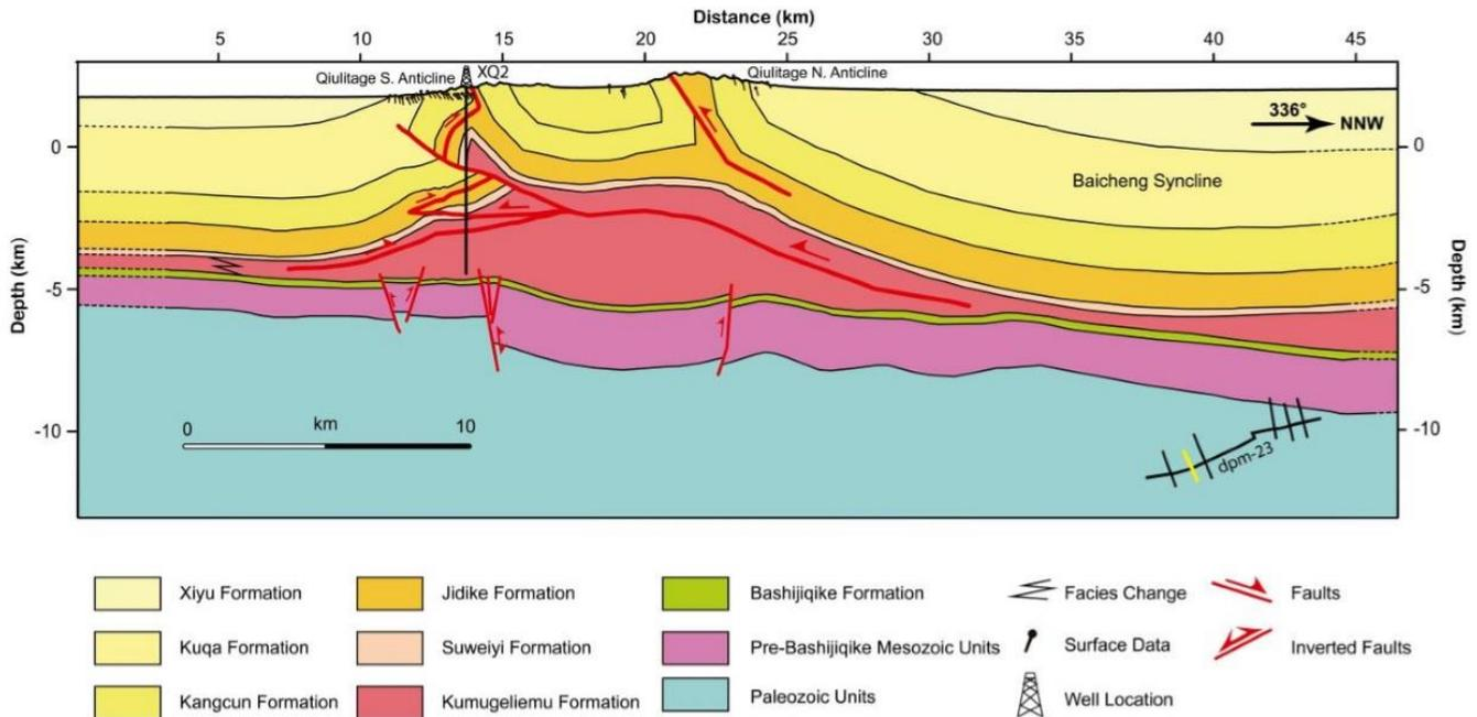
**Figure 2.** Cross-section interpretation of depth-converted 2D seismic profile Short 4, including the position of Well DQ2.
