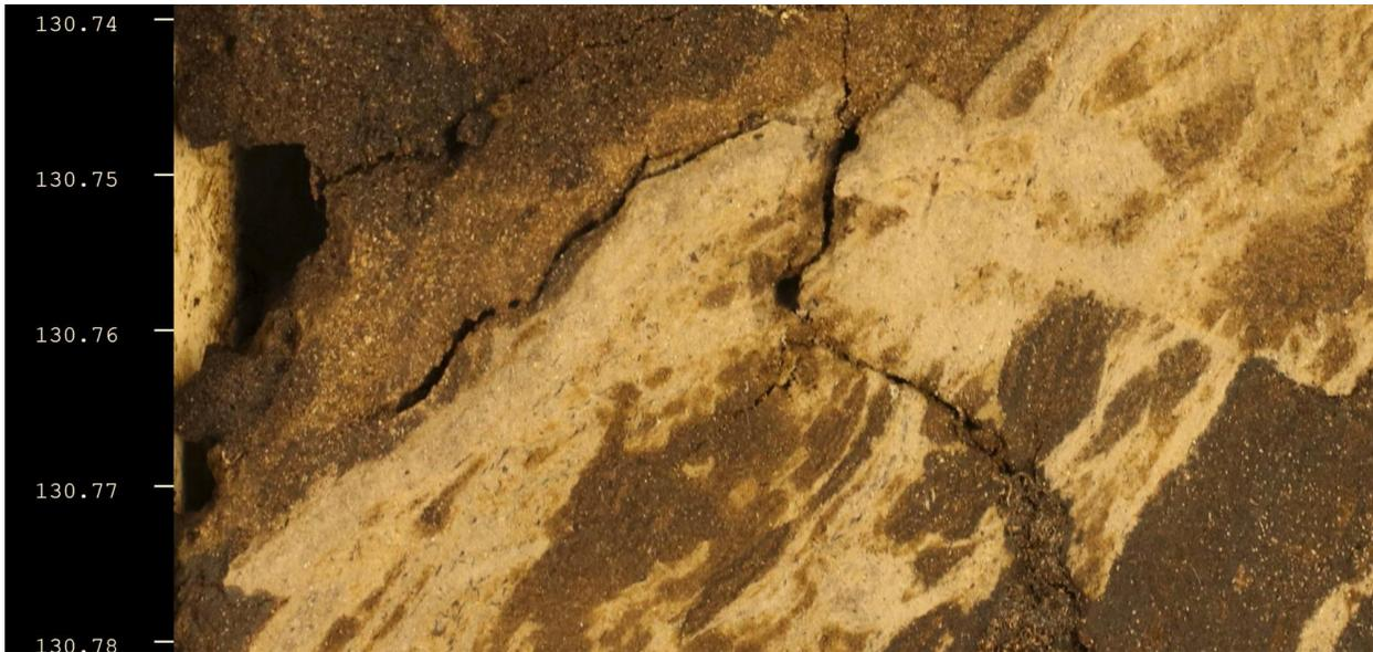
Figure 1: A high resolution RGB image of a dipping mud laminae which contains trace fossils filled with bitumen stained sands, a small fault, a sharp base and a more defuse top with a gradual change in mud content. The scale on the left is in centimeters.
