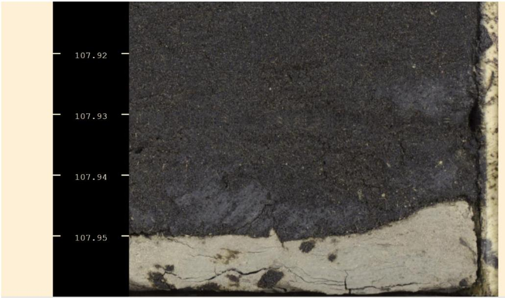
Figure 2: The mud laminae at the base of the bitumen saturated sands has scattered trace fossils, sharp top and bottom contacts, and internal silt and sand grains which are laminated.
