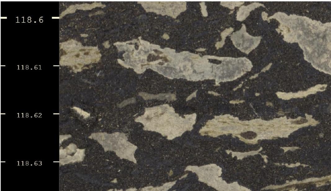
Figure 3: An image of mud breccia in a fine-grained bitumen-saturated sand. Note that the clasts are not touching, angular, partly bioturbated, and appear coarsely bedded.
