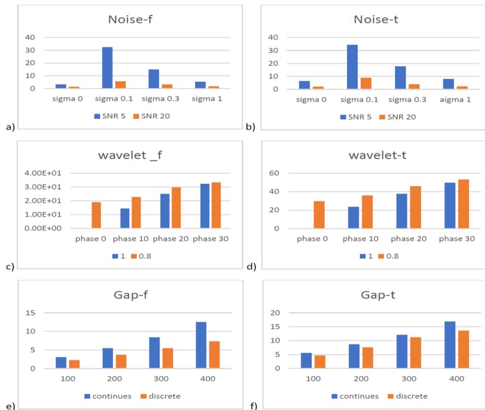
**Figure 3.** Error calculated from equation (1), (a) frequency domain FWI result with noise error, (b) time domain FWI result with noise error, (c) frequency domain FWI result with source wavelet error, (d) time domain FWI result with source wavelet error, (e) frequency domain FWI result with gap, (f) time domain FWI result with gap.
