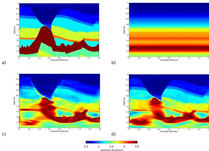
**Figure 1.** (a) True velocity model. (b) Initial velocity model. (c) noise free FWI result for frequency domain. (d) noise free FWI result for time domain.
