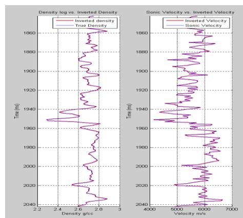
Figure 1: well log velocity (left, blue) and inverted velocity (left, red); well log density (right, blue) and inverted density (right, red)
