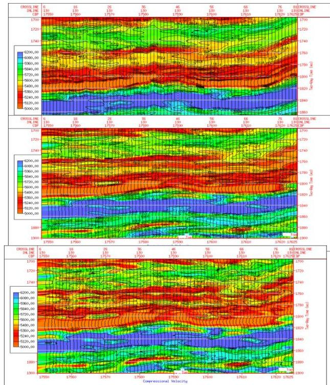
Figure3: The velocity inversion using different sample rates (top 1ms, middle 0.5ms and bottom 0.25ms) based on our Bayesian-based Support Vector Machine geostatistical inversion.
