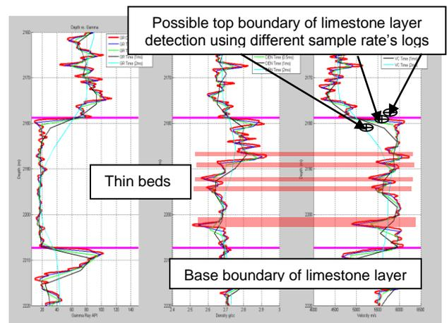
Figure 2: well logs and their responses with different sample rates.
