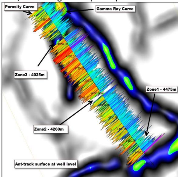
ray response. These intervals would not complete well, all the energy would travel along the fracture and not break new rock. In addition, energizing these fractures during the completion could cause the rock faces to slip, leading to 'crimping' of the well casing. Missing out selected sleeves over these intervals therefore gives us both better well productivity and better capital efficiency
