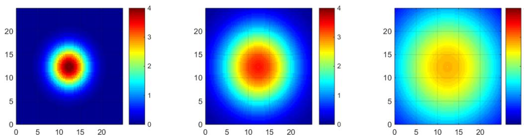
Figure 1: The pore pressure transient around a constant temperature steam injection well calculated for (from left to right) 6 months, 2 years and 5 years of continuous operation. Colour scale is in MPa and axis distances in metres.
