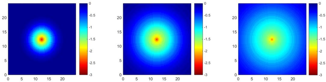
Figure 2: The change in P-velocity surrounding a steam injection well calculated for (from left to right) 6 months, 2 years and 5 years of continuous operation. Colour scale is in percent and axis distances are in metres.
