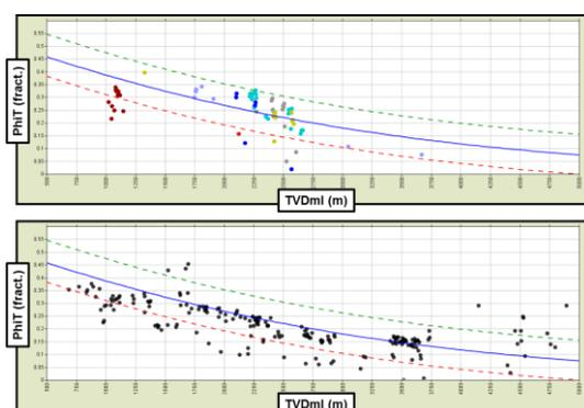
Figure 1: Porosity (PhiT) - depth (TVDml) trend for clean sandstone. The upper plot shows the data from the Flemish Pass and Orphan Basins, the lower is analogue data from mid Norway. The blue trend is the mid-point porosity case, the green is the high porosity case, and the red the low porosity case.
