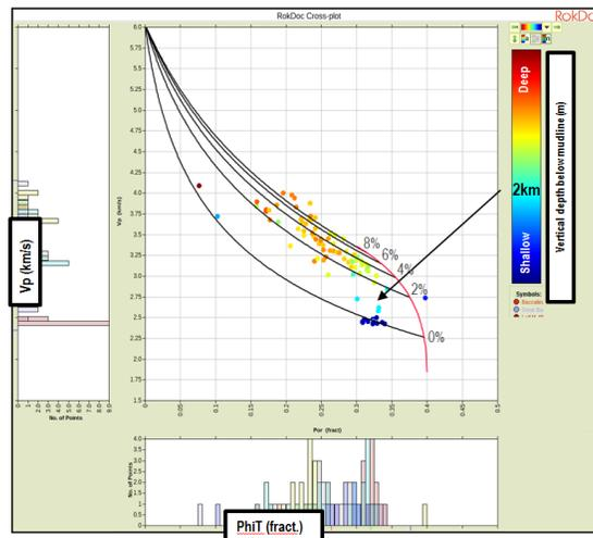
Figure 2: Velocity-porosity responses for clean sandstones in the study wells, coloured by burial depth. The blue line is the unconsolidated sandstone lines, the grey lines are lines of constant grain contact cement.
