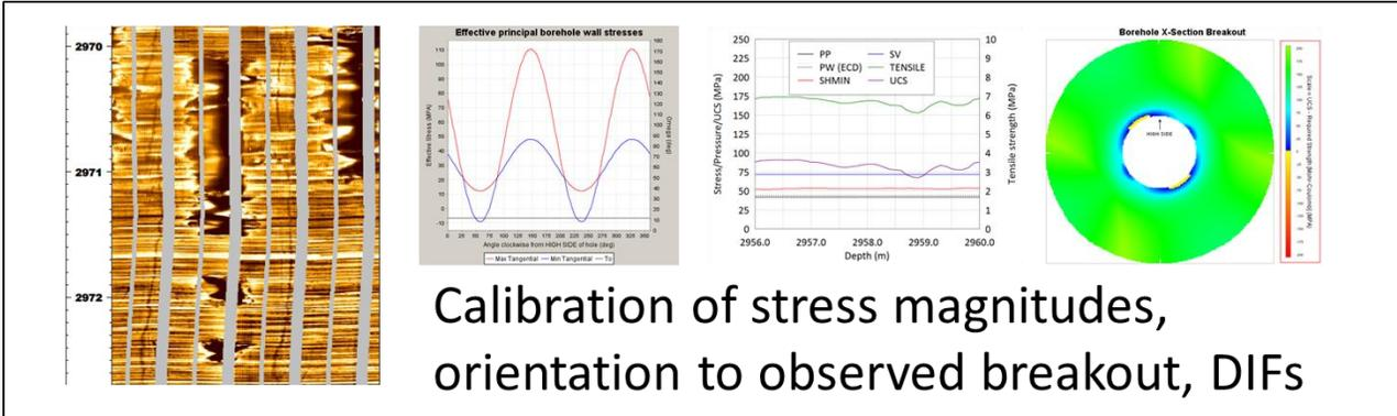
Calibration of stress magnitudes, orientation to observed breakout, DIFs
