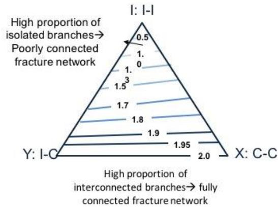
Figure 3. Branch behaviour leading to assessment of the potential for percolation.
