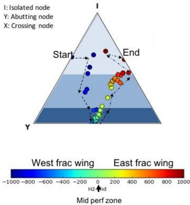
Figure 4. Topologic mapping of the fracture network with position relative to the treatment zone for one stage. Three zones are defined based on the observed interconnectivity of the network, suggesting a gradational variation in fracturing behaviour with position from the treatment zone, in-line with the concept of trilinear models.
