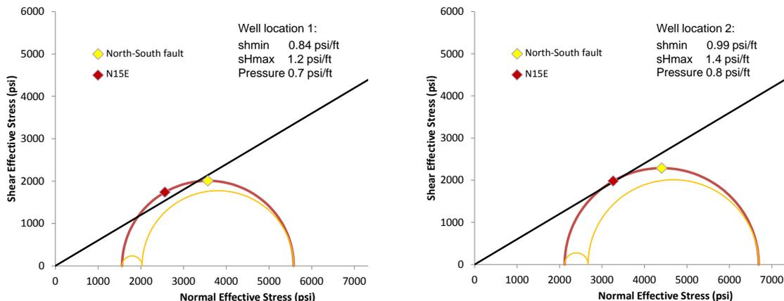
Fig. 1. Mohr circle plots for effective stress state at two sample well locations in Duvernay. The initial stress state is close to shear failure and small stress/pressure perturbations may cause fault slip. Faults oriented N15E are more likely to slip first. Faults assumed to have friction coefficient of 0.6 and negligible cohesion.
