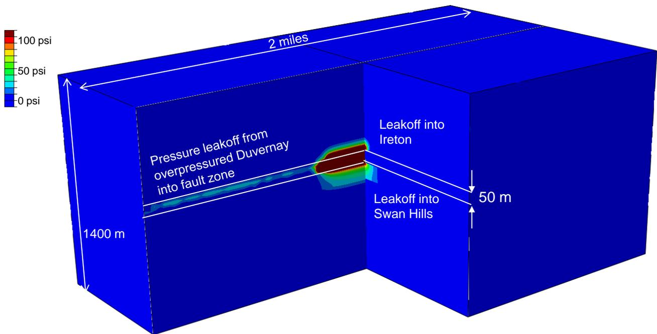
Fig. 4. Excess pressure after 10 days due to pressure diffusion along fault zone and surrounding layers due to fault-fracture intersections; 15 fractures held at pressure of constant  $sh_{min}+500\text{psi}$ , fault zone 1m wide with 1 millidarcy permeability
