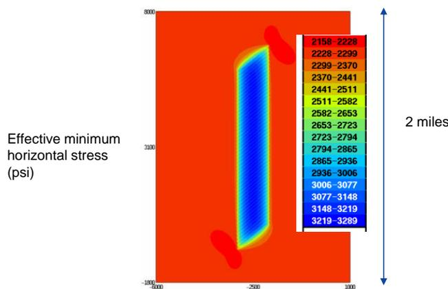
Fig. 2. Effective minimum horizontal stress with changes induced by fracture pressure; stress changes attenuate quickly away from fractures.
