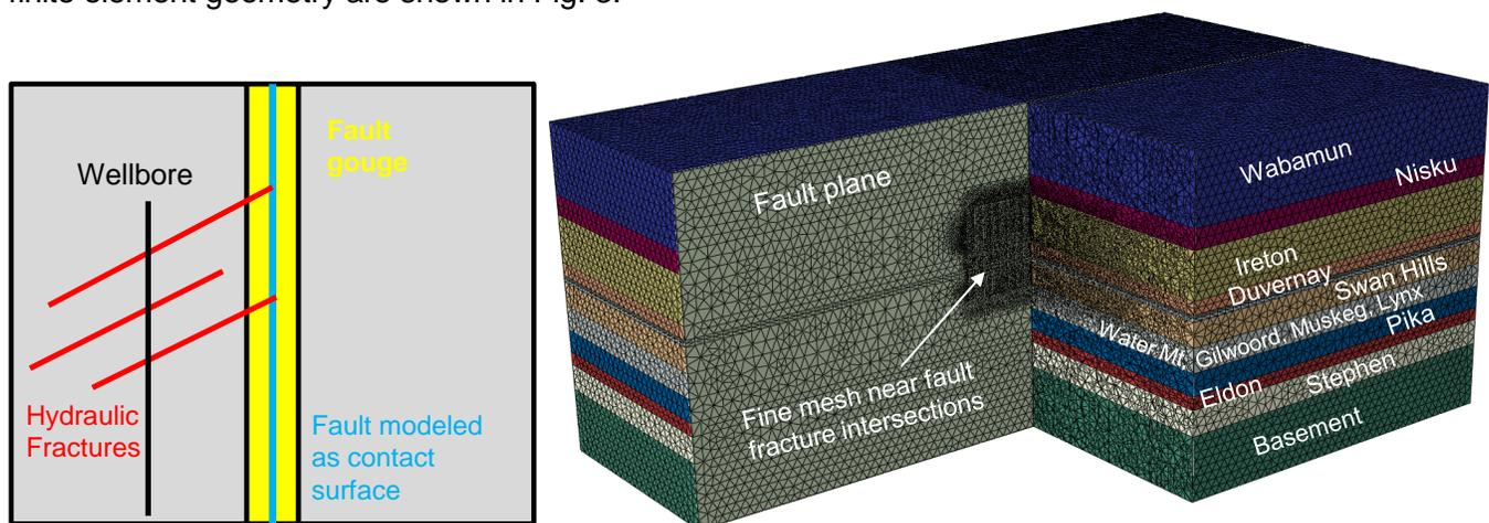
Fig. 3. Schematic plan view of fault-fracture intersection with North-South fault and North-South horizontal wellbore; details of 3D finite element model with geological layers and mesh
