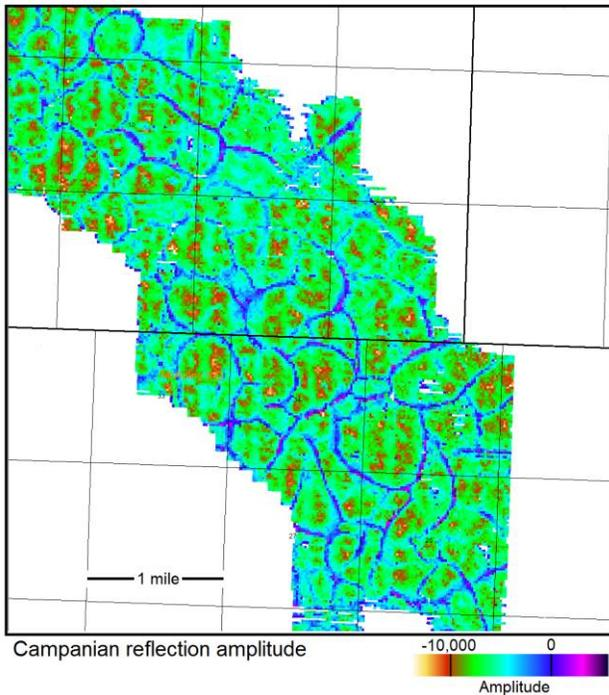
Figure 5 – Campanian Lea Park amplitude reflection for a confidential 3-D survey acquired in Manitoba near the Saskatchewan border approximately at Twp 15. The low amplitude areas map arcuate fault traces that have ~15 m of vertical offset in the Lea Park beds.
