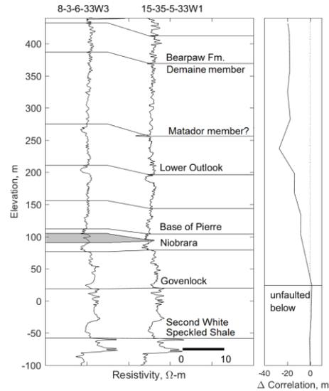
Figure 4 – Two well cross section from southeast Saskatchewan a missing ~20 m of section in the Niobrara Formation. And the fault timing based upon correlative markers in the two wellbores.
