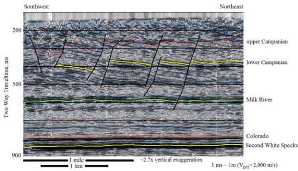
Figure 3 – Two dimensional seismic line from southeast Saskatchewan showing faulted Upper Cretaceous sediments. The 200 ms time is ~ 200 m below ground surface. The deeper reflection from Colorado Formation strata and deeper are unfaulted
