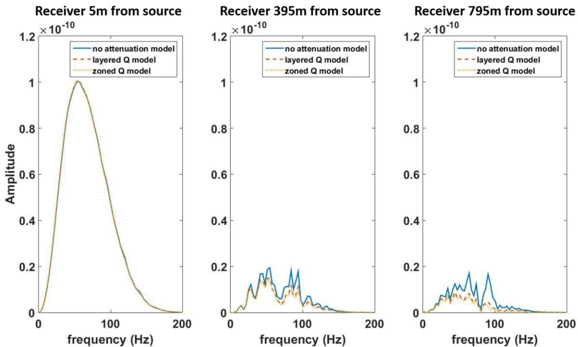
Figure 5 Amplitude spectra of different Q configurations at various receiver locations
