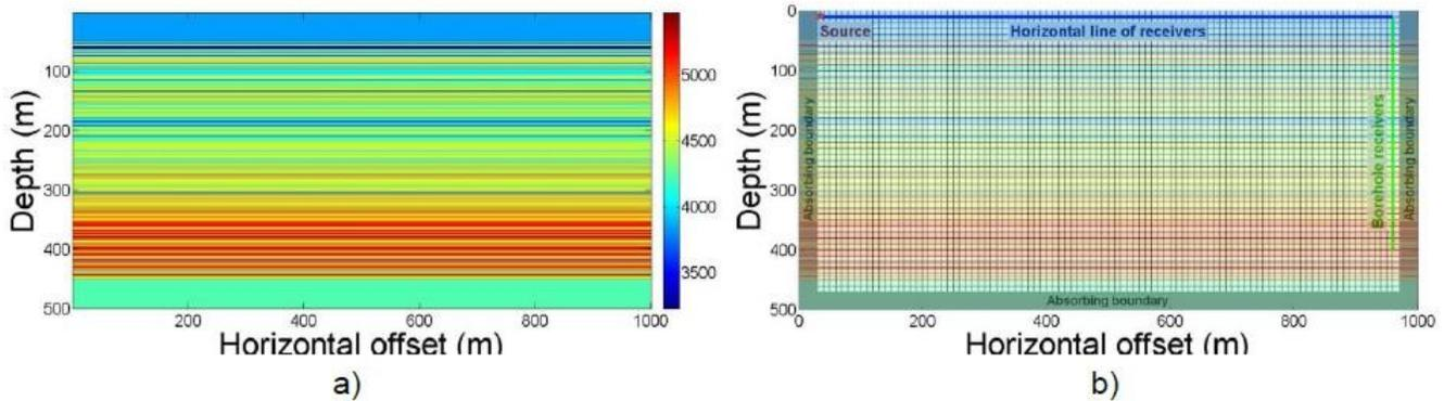
**Figure 1 a) Athabasca velocity structure (m/s); b) model geometry**
