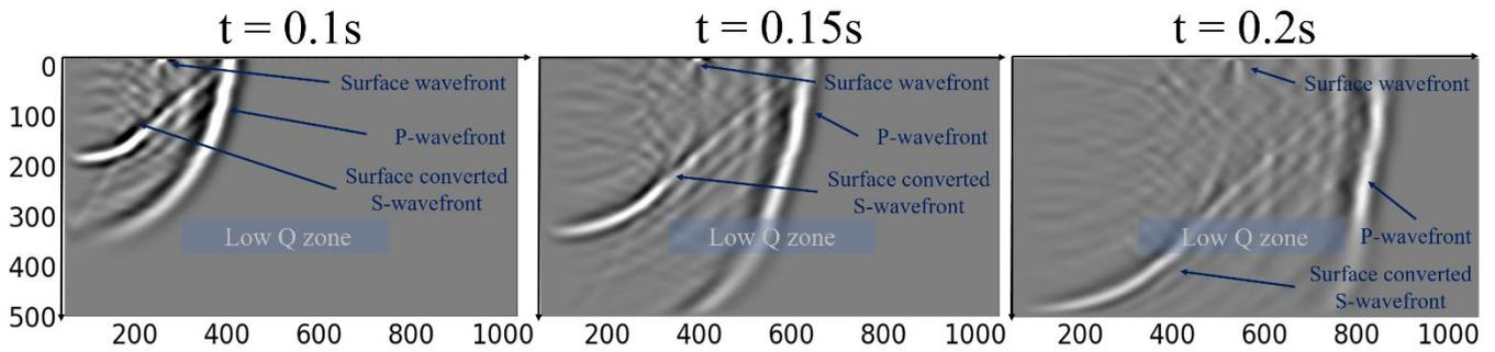
**Figure 3 Snapshots for x component wavefield in localized attenuation model**
