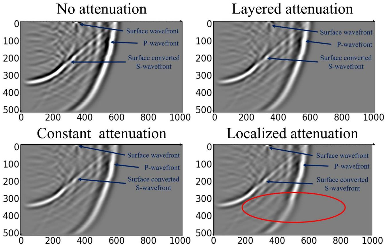
**Figure 4 Snapshots of wavefield of different Q structures at t = 0.15s**
