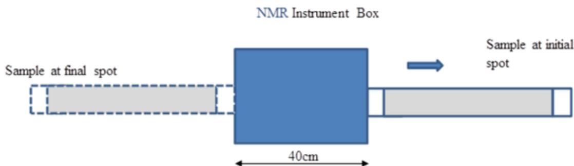
**Figure 1.** Illustration of NMR measurement process for core logging.
