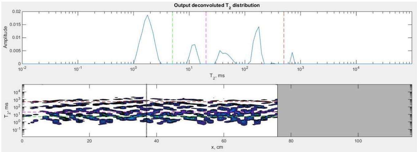
**Figure 5.** Downscaled  $T_2$  distribution along the core. The top panel shows  $T_2$  distribution for one position along the core. The bottom panel presents  $T_2$  distributions for all positions along the core.
