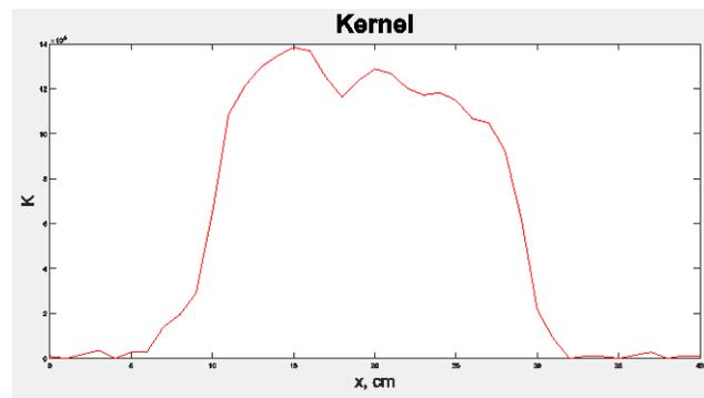
**Figure 3.** Example of estimated kernel from Step 1 for water sample. The resolution of the kernel is  $\delta = 1$  cm. The length of the kernel is  $\Delta = 40$  cm. Sweet spot for the kernel contains about 20-23 cm. Outside of this interval the signal is very small.
