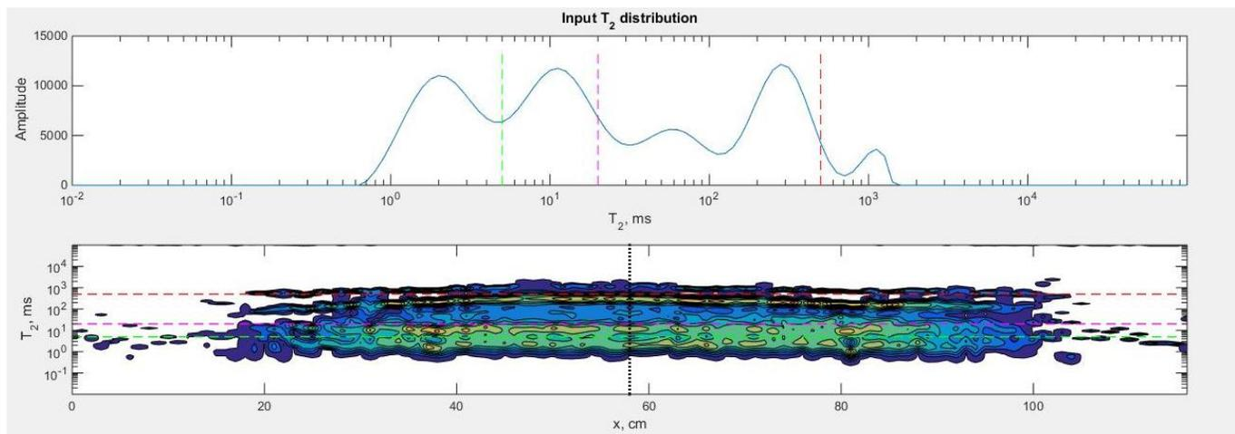
**Figure 4.**  $T_2$  distribution along the core measured using NMR instrument with kernel of length 40cm shown in Figure 3. The top panel shows  $T_2$  distribution for one position of the core in the NMR instrument. The bottom panel presents  $T_2$  distributions for all positions in the NMR instrument.
