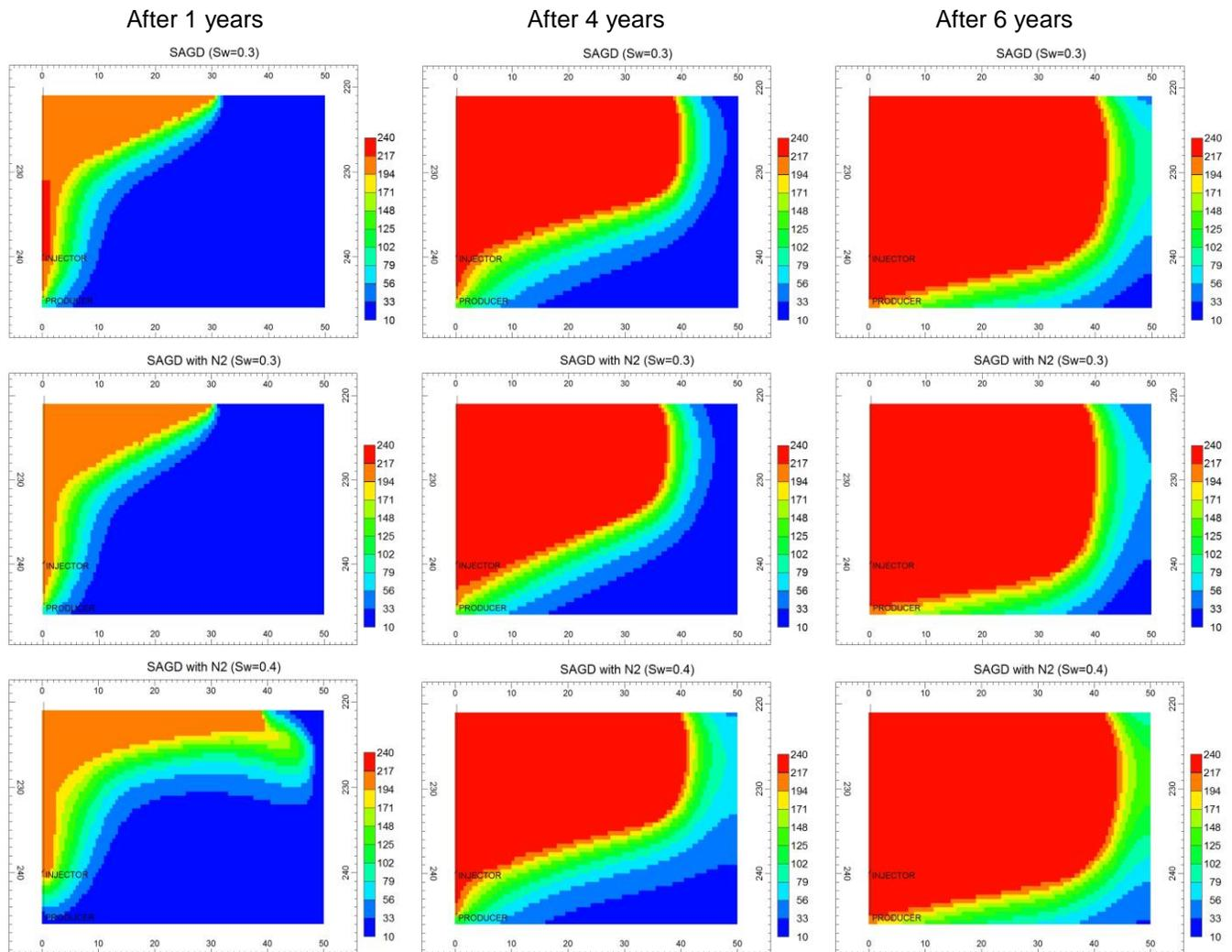
Figure 2 Variation of steam chamber with time
