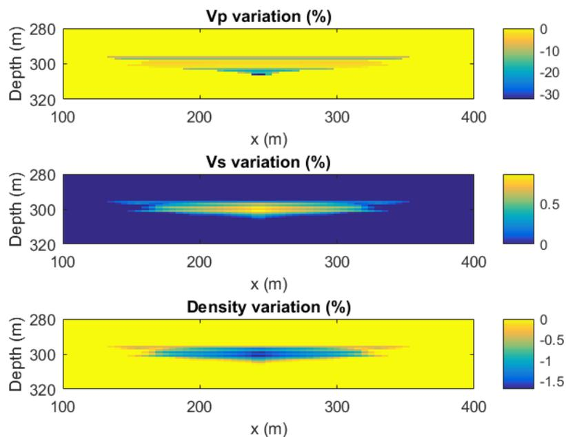
**Figure 2.** 2D sections in the variation of elastic parameters for  $t=6$  year, focussed on the  $\text{CO}_2$  reservoir injection. Top: P-wave velocity variation. Middle: S-wave velocity variation. Bottom: Density variation.
