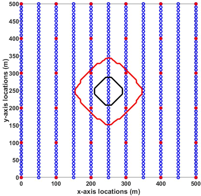
**Figure 1.** Maximum extension of the CO<sub>2</sub> injection plume (depth = 296m), 1 year after the beginning of the injection (in black) and 1 year after the end of the injection (in red). Surface survey configuration for the seismic simulation is added; blue squares are receivers, red crosses are sources.
