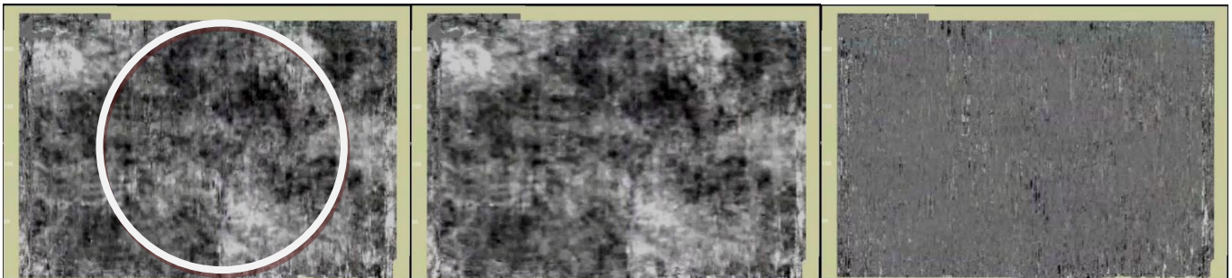
Figure 3: Left is the 5D only interpolated stack timeslice in the shallow, middle is the cascaded 2D and 5D interpolated stack timeslice and far right is the difference. The cascaded interpolation shows a clearer image as it better handles the vertical aliasing/acquisition footprint noise as shown.
