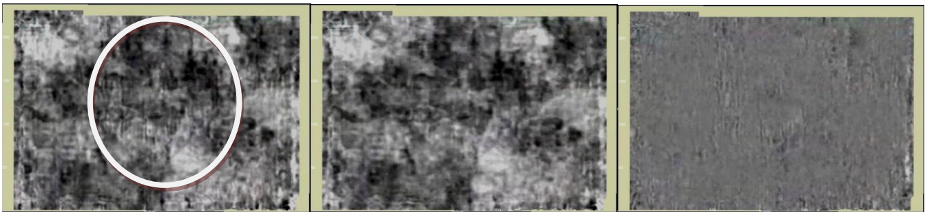
Figure 7: Left is the 5D only interpolated PSTM stack timeslice in the shallow, middle is the cascaded 2D and 5D interpolated PSTM stack timeslice and far right is the difference. The cascaded interpolated timeslice shows a clearer image with less vertical footprint/aliased noise as highlighted.
