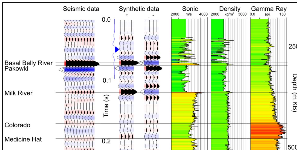
Figure 1: Migrated PP seismic data tied to normal incidence synthetic seismogram. Notice the poor character match at the Milk River.
