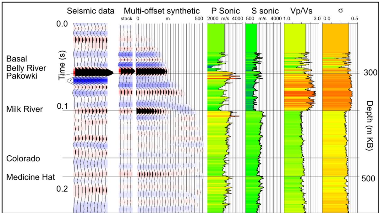
Figure 2: Migrated full-offset seismic data tied to stacked offset synthetic seismogram. Notice the improvement in the tie at the Milk River compared that of the normal incidence synthetic seismogram in Figure 1.
