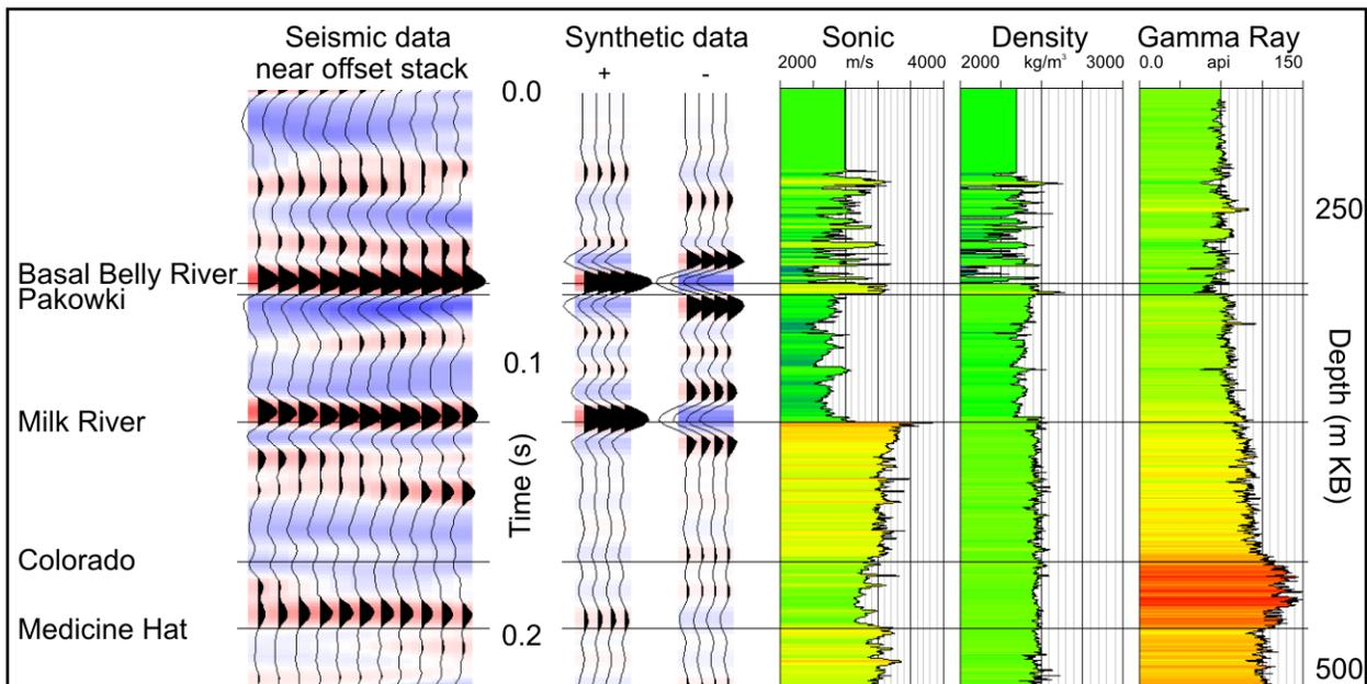
Figure 3: Migrated limited-offset seismic data tied to normal incidence synthetic seismogram. Notice the improvement in the character match at the Milk River compared to that of the full offset migrated seismic data in Figure 1.
