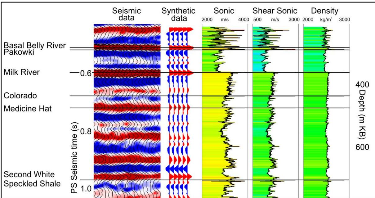
Figure 4: Migrated PS seismic data tied to the PS synthetic seismogram.
