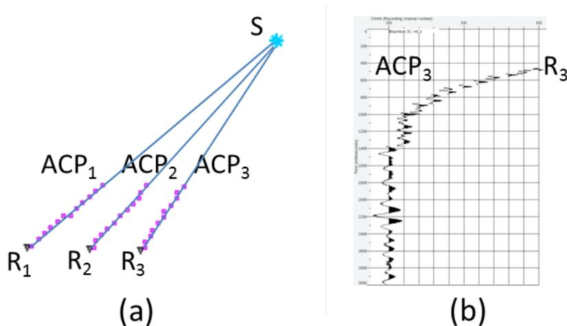
Figure 3. CCP binning example on CREWES 3C-3D data. (a) Shot-receiver geometry for three receivers. (b) Trace split into CCP bins for receiver  $R_3$ .
