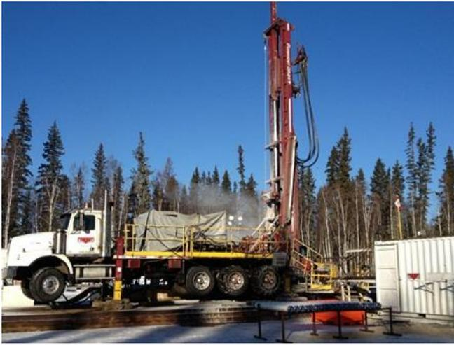
Figure 1 – Mud rotary coring rig adapted for 6” coring and wireline core retrieval.
