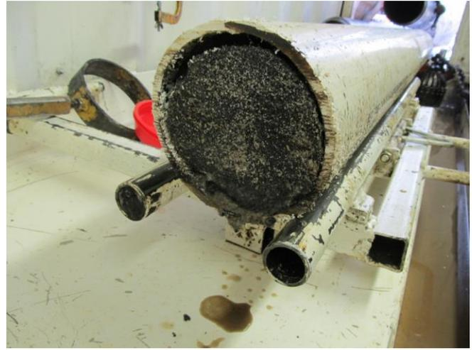
Figure 2 – Example of oil sands core inside 6” PVC tube.
