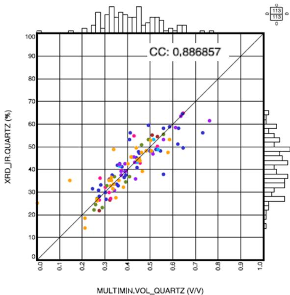
Figure 7. Linear regression analysis of Quartz demonstrated strong correlations between of the probabilistically determined parameters for 53 wells to core analysis data. R2 =0.89
