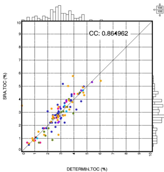
Figure 8. Linear regression analysis of TOC demonstrated strong correlations between of the Passey-Schmoker determined parameters for 53 wells to SRA analysis data. R2 =0.86
