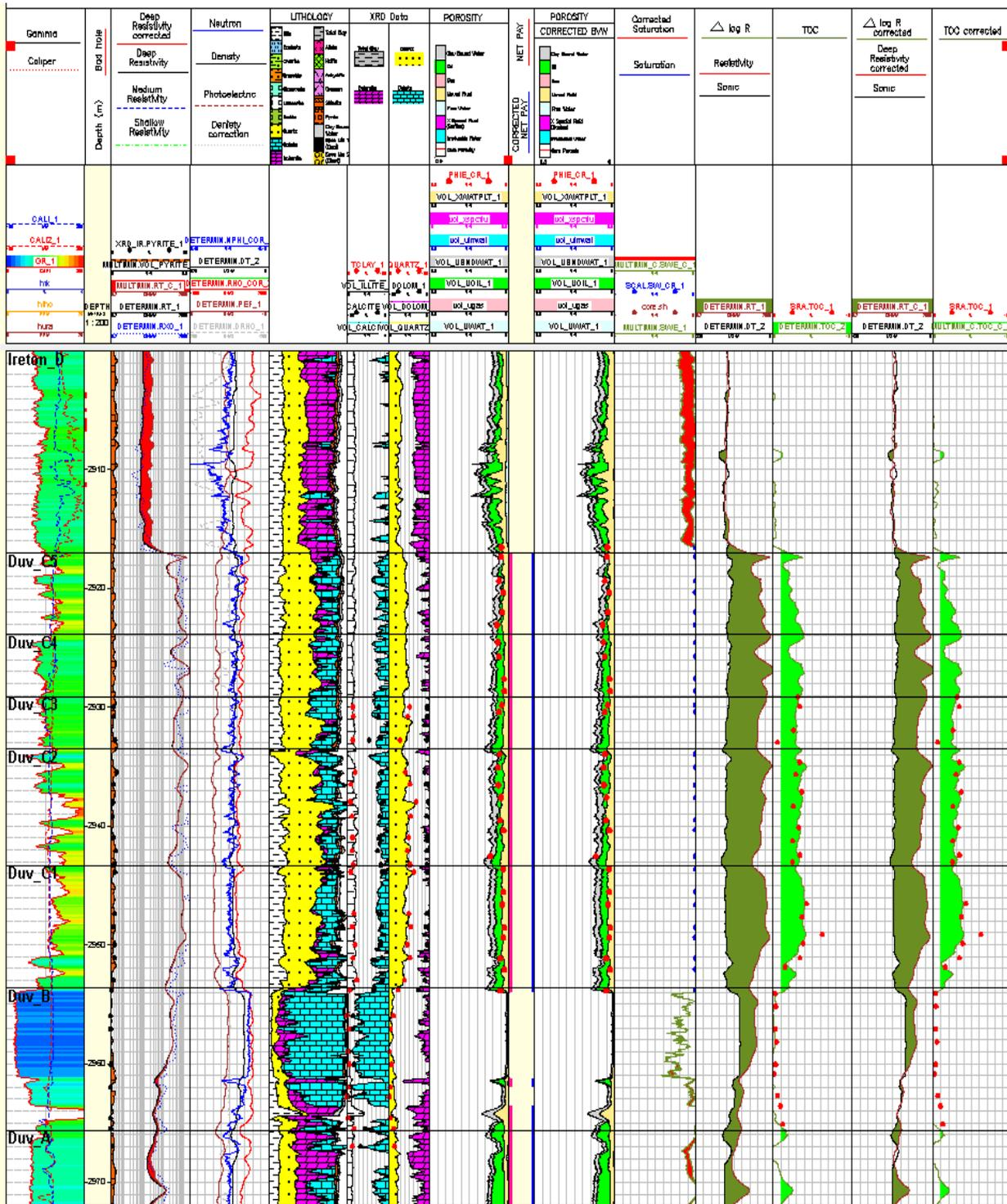
Figure 6 (Example 4).. Duvernay: Probabilistic Petrophysical Analysis and Passey Schmoker TOC displaying good correlation with XRD mineralogy and SRA TOC. Comparison of analyzed  $S_w$  and TOC after pyrite correction.
