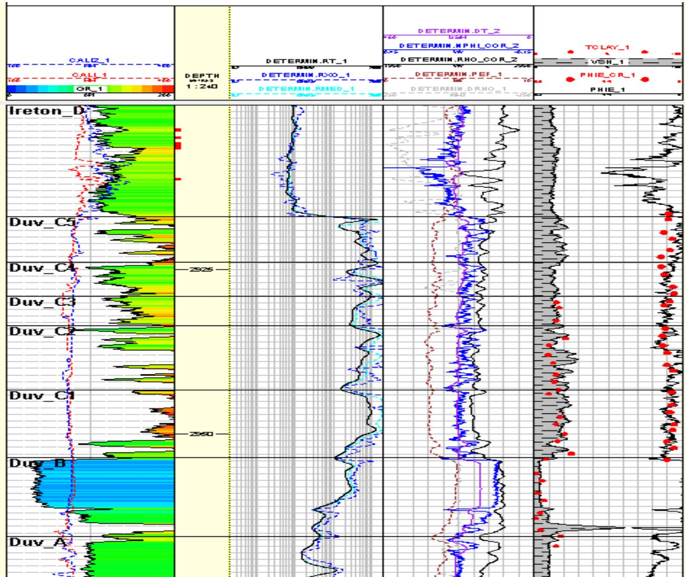
Figure 3 (Example 1). Calculated  $V_{sh}$  and  $\Phi_{eff}$  showing good correlation with XRD Total Clay Volume and effective core porosity
