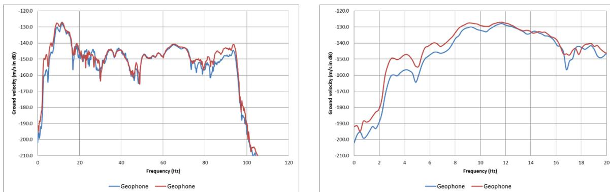
Figure 3: Ground velocity vs. frequency for two separate lines of geophones. (Left) Complete response. (Right) Zoomed in to 0-20Hz.
