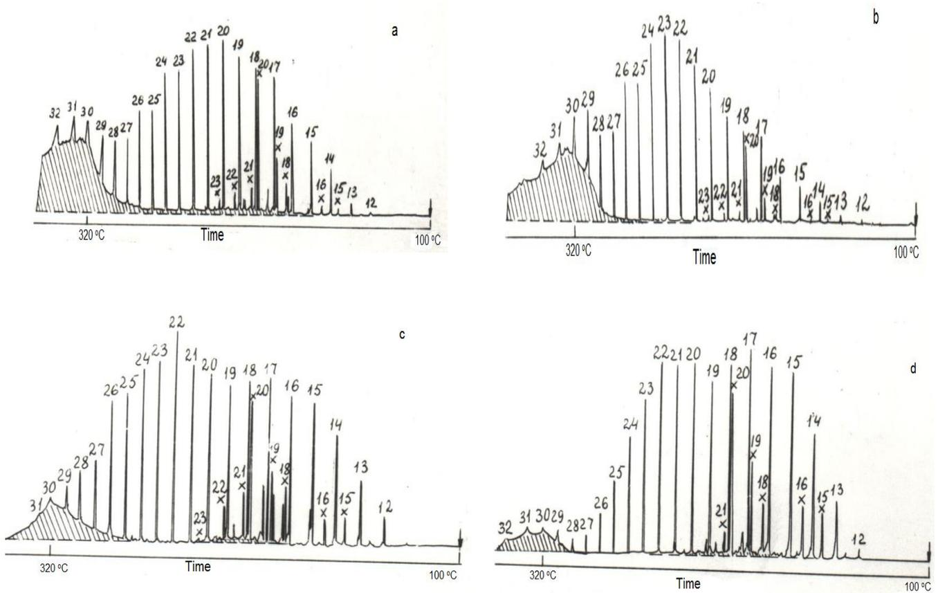
Fig.3. Gas chromatograms of oils extracted from samples of carbonate rocks: 1 - extracted oil, 2, 3, 4 – condensates of steam displacement of oil at 500, 400 and 300 °C, respectively.
