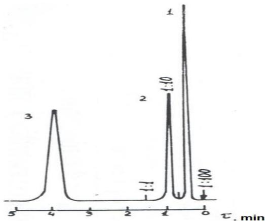
Fig. 1 – A typical chromatogram of gas releasing from carbonate rock at 350 °C:
