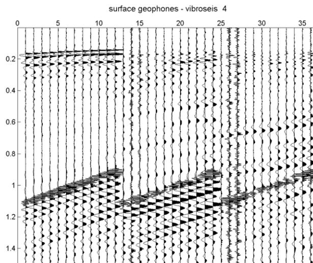
Figure 6: Vibroseis data recorded from conventional surface three-component geophones with identical elements for comparison.
