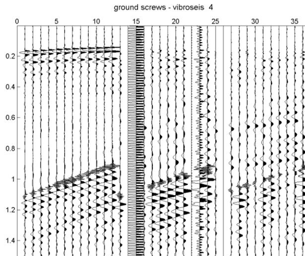
Figure 5: Vibroseis data recorded from geophones installed in ground screws. The missing and noisy traces are obvious, but the high frequency air-blast noise is less than in the conventional record.
