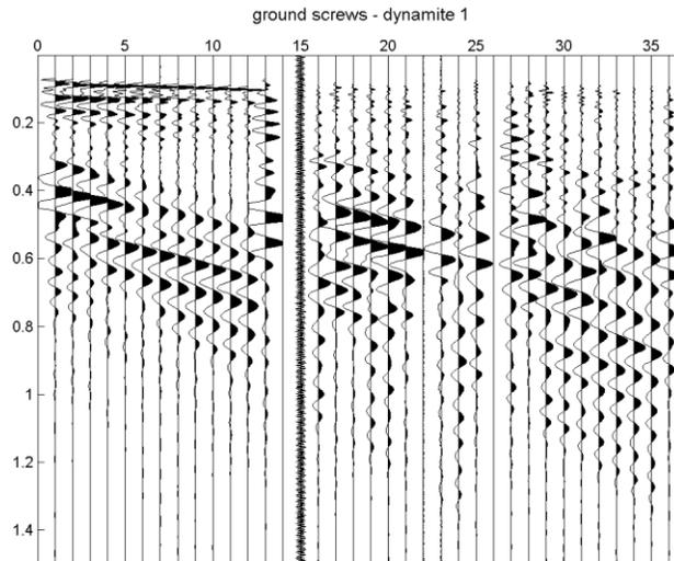
Figure 3: Dynamite data recorded from geophones installed in ground screws. There are 12 traces each of vertical data, in-line horizontal data, and cross-line horizontal data. There are several missing and noisy horizontal traces.
