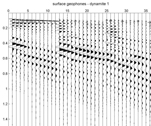
Figure 4: Dynamite data recorded from conventional surface three-component geophones with identical elements for comparison.
