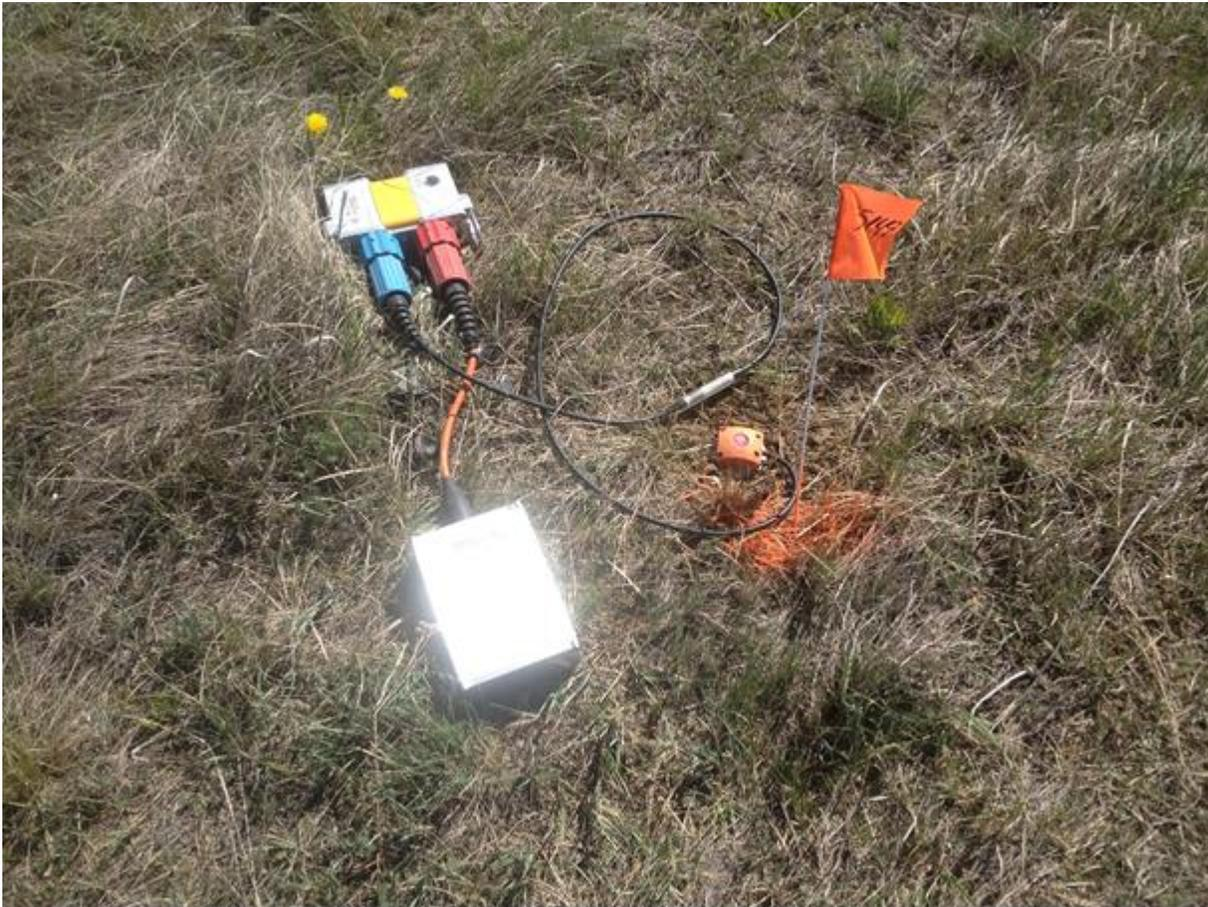
**Figure 1:** An example of a typical wireless recording station consisting of one battery, one recording unit and one battery. A system like this HAWK unit is capable of recording for 20-30 days depending on temperature and daily recording hours.
