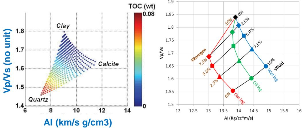
**Figure 2 Sensitivity analysis of geophysical properties (AI & Vp/Vs); the left plot shows changes with mineral and TOC content (Zhu et al, 2010); the right plot shows changes with kerogen and fluid content for a constant porosity (10% total porosity) unconventional reservoir (Malaver, 2014). Pore pressure or geopressure will affect both Vp/Vs and AI.**
