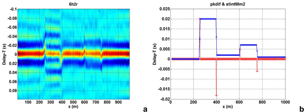
Figure 3. (a) Stacked crosscorrelations for each receiver. Notice the time delay at the limit between the lateral zones of Fig. 2. (b) Differential delay  $\delta R$  after the result of Fig. 3(a) according to Eqn. 3, shown by red crosses, and statics calculated from the differential according to Eqn. (4) shown by the blue line with dots.
