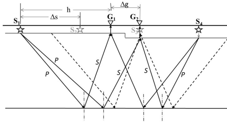
Figure 1. The *PS*-wave events that arrive at two adjacent receivers ( $G_1$  and  $G_2$ ) with a differential time delay  $\delta R$  (statics) between them, illustrated by raypaths. The events generated by different sources ( $S_1$  and  $S_4$ ) should have the same differential delay  $\delta R$ . However there is an additional delay generated by the different offset  $h$ . The dashed rays, however, have the same offset, and interpolation is proposed to obtain them.
