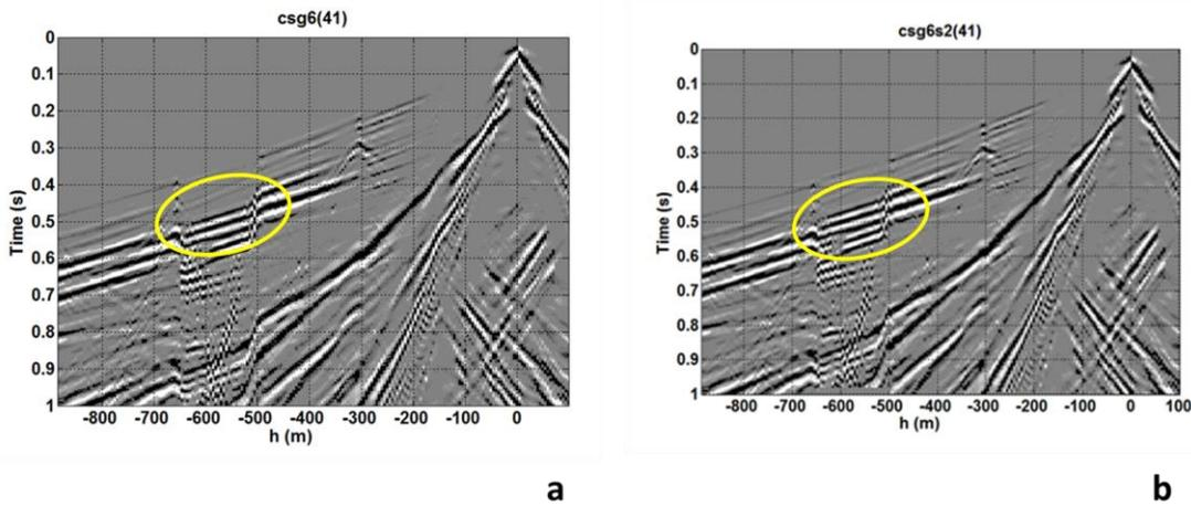
Figure 4. Seismic data in the source domain after the application of the receiver statics correction of Fig. 3(b). (a) Before statics, (b) after receiver statics application. Notice the improved continuity of the events.
