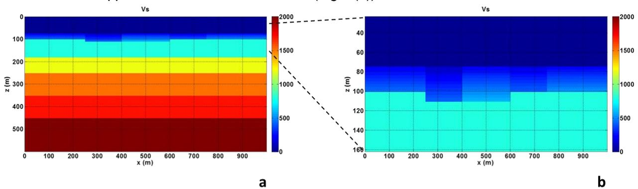
Figure 2. Synthetic model: (a) S-wave velocity model. The free surface is at  $z=75$  m. (b) A close-up of the near surface. Notice the lateral velocity variation in five zones and a depth velocity gradient.
