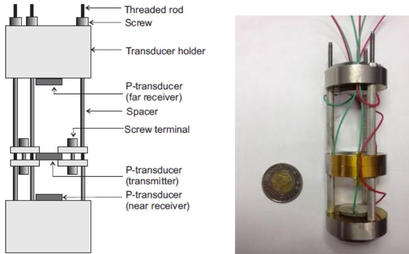
**Figure 1:** Pulse-transmission approach for highly attenuating fluids consisting of a central single transmitter and far and near receivers. Left - the schematic of the cell and right picture shows the actual cell made with stainless steel.
