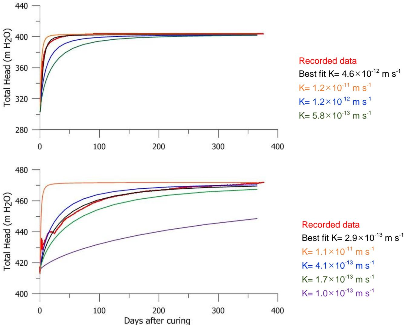
**Figure 2:** Measured and simulated total hydraulic head recovery for two transducers (B and E). Transducer B illustrates the characteristic recovery trend of the deep transducers (225-325 m BG) and Transducer E illustrates the characteristic recovery trend of the shallow transducers (50-185 m BG).
