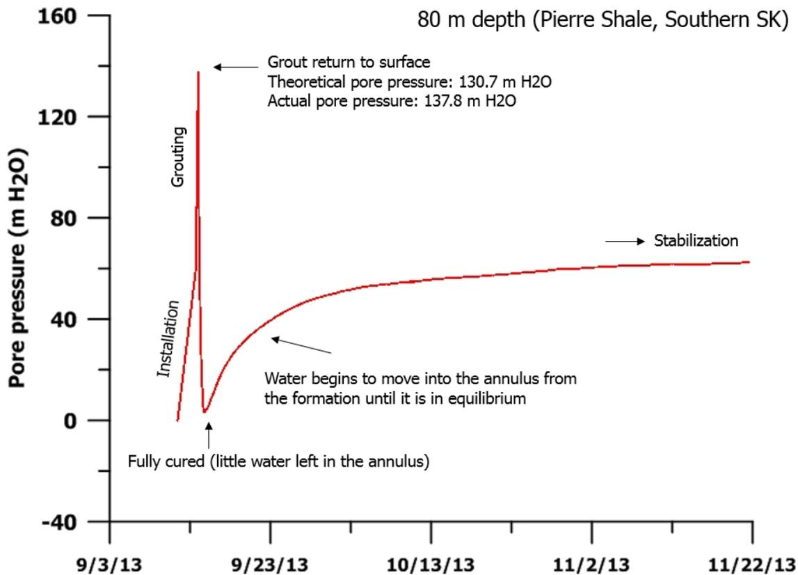
**Figure 1:** Typical pore pressure response after grouting in a pressure transducer.
