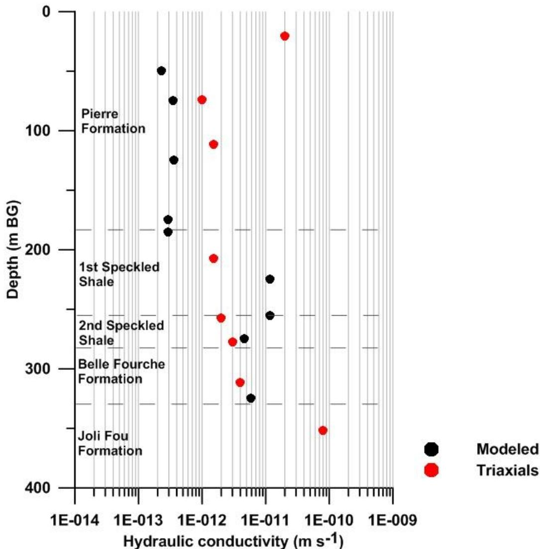
Figure 3: A comparison of laboratory and *in situ* results for estimated K.
