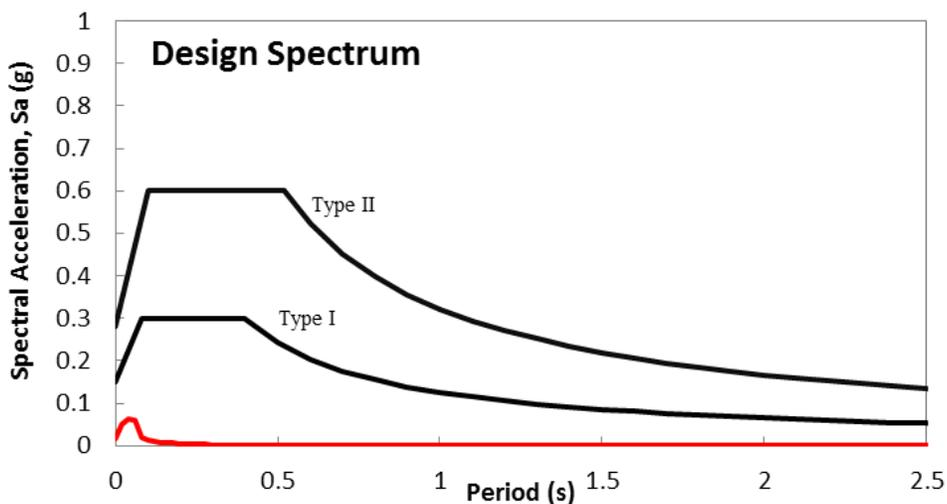
Figure 4. Red line is the response spectrum related to the Mw2.9 events in relation to the building code specifications related to the UBC-97 design spectra for difference soil and subsurface conditions.
