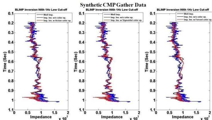
Figure 4. The result of Impedance inversion with BLIMP for different color operator (low cut-off frequency=1Hz).
