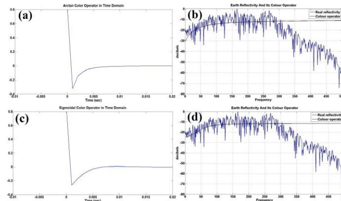
Figure 2. Minimum phase color operator derived from well reflectivity. (a) the Arctan color operator and (b) its amplitude spectrum in frequency domain, (c) the Sigmoidal color operator and (d) its amplitude spectrum in frequency domain.
