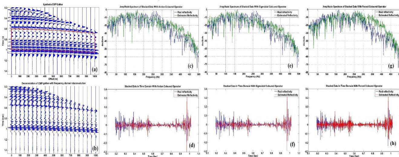
Figure 3. The effect of color operator in reflectivity estimation from synthetic CMP gathers (a), deconvolution of synthetic CMP gathers (b), amplitude spectrum of stacked data resulted from applying arctan color operator (c), stacked data for same color operator in time domain (d), (e) and (f) the same results with applying sigmoidal color operator, (g) and (h) with applying forced color operator.
