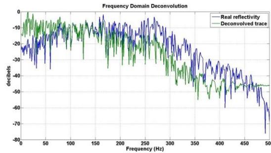
Figure 1. The effect of frequency domain deconvolution with white spectrum assumption on deconvolved data.
