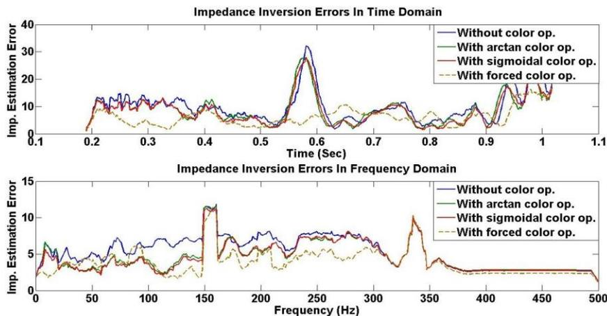
Figure 5. Effect of color operator on impedance estimation errors in time and frequency domain (synthetic shot gather data).
