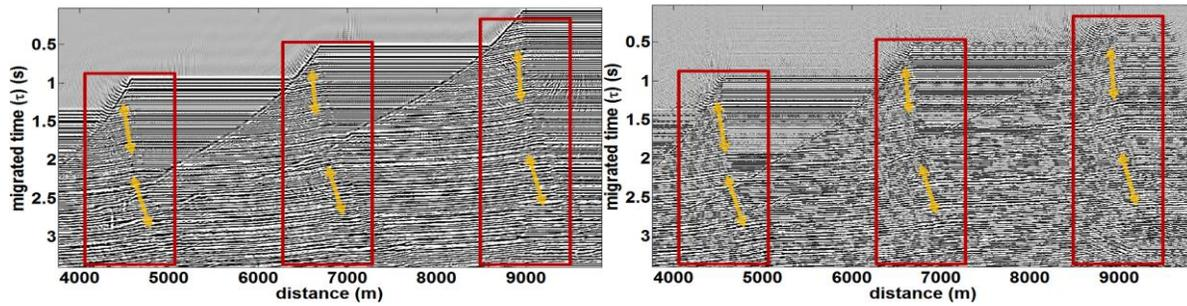
FIG.3. (left) Poststack time migration of exploding reflector model and (right) Poststack time migration of common midpoint stacked section
