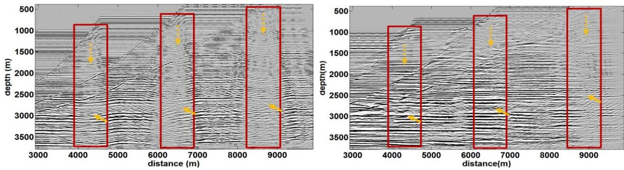
FIG.6. (left) Iterated poststack depth migration and (right) Iterated prestack depth migration with fault constrained velocities
