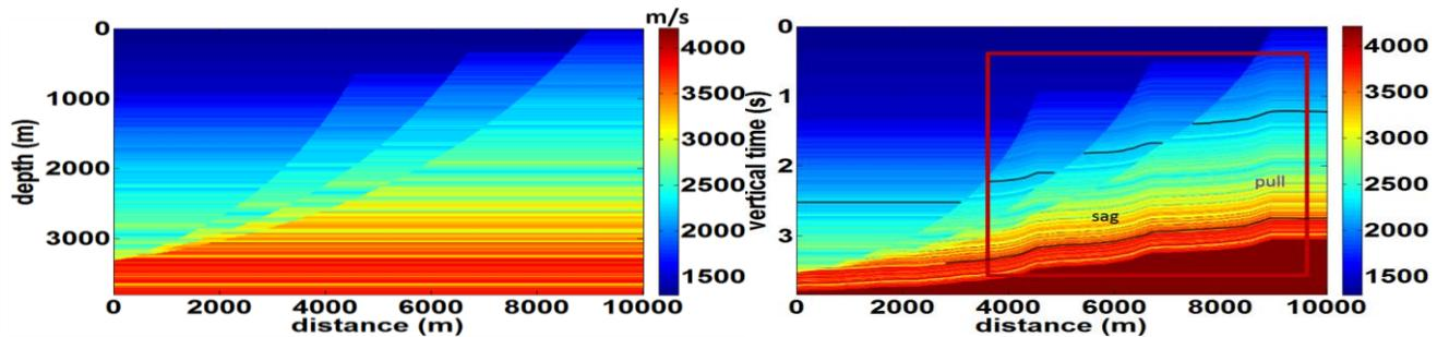
FIG.1. (Left) True geologic model (top) and two-way time velocity model and (right) obtained from depth to time computation. Time distortions behind the fault extends into the footwall of faults and appears as time pull up and sags.
