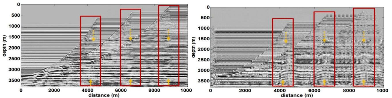
FIG.4a. (left) Poststack depth migration of exploding reflector model with true velocity and (right) Poststack depth migration of common midpoint stacked section with true velocity.
