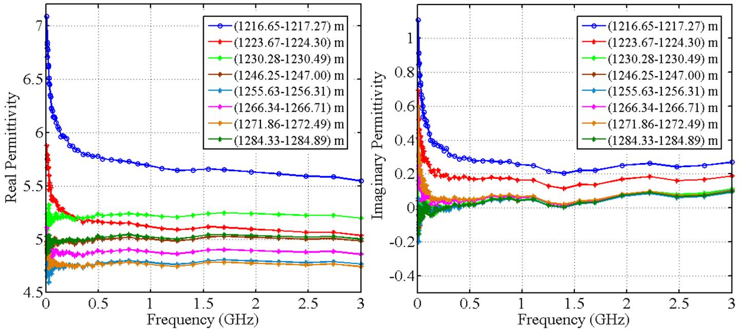
Figure 1: The real and imaginary permittivity of samples taken from GPR reflection zone. The samples names stand for the depth it was taken from.
