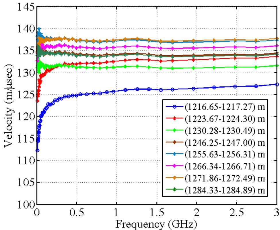
Figure 2: The velocity of samples taken from GPR reflection zone. The name of the samples stand for the depth it was taken from. At high clay content the velocity becomes a function of frequency.
