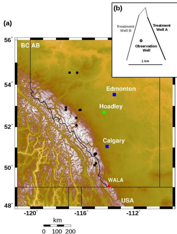
**Figure 1.** (a) Map showing locations of regional earthquakes, detected using a downhole geophone array at Hoadley. (b) Inset shows layout of the treatment and observation wells.
