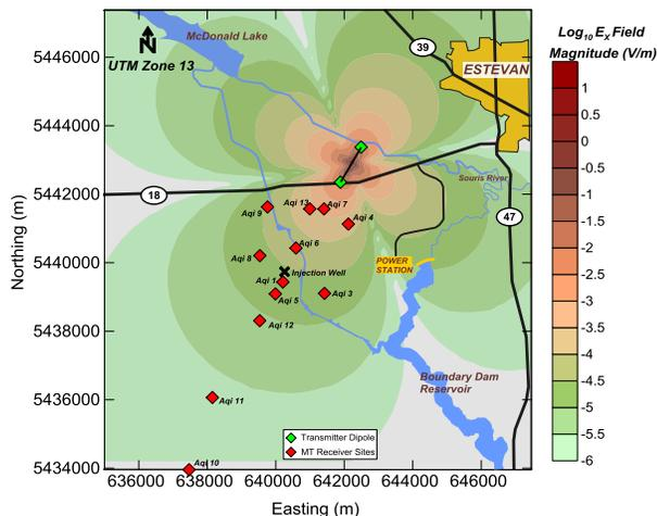
**Figure 3.** Signal pattern produced by an electric dipole source at the Aquistore site. Contours show the component of total electric field parallel to the source.
