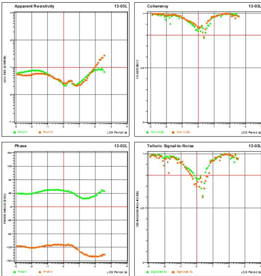
**Figure 2:** MT responses for aqi 05 for 2013 survey. Left panels show apparent resistivity and phase responses. Green curve is the xy-component (north-south electric current) and orange curve is the yx-component (east-west current). Right panels show measures of EM noise: local Ex-Hy and Ey-Hx coherences and telluric signal-to-noise ratio.
