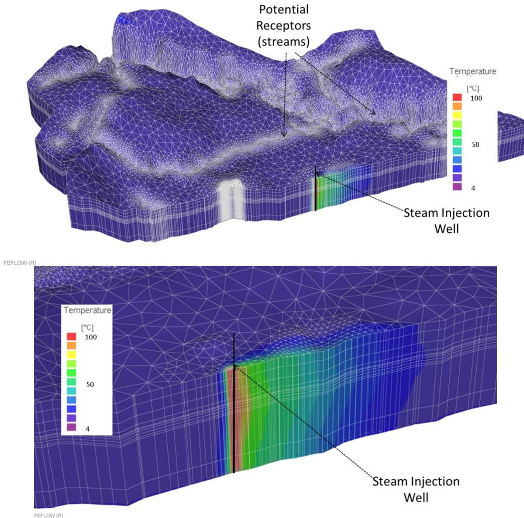
*Model of a thermal plume from the vertical portion of a SAGD wellbore within 3D finite element groundwater model built in Feflow. Groundwater model was based on site specific subsurface geological and hydrogeological characterization and surface topography.*
